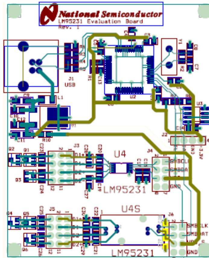
Figure 5.3 Layout diagram of the LM95231 Evaluation Board
