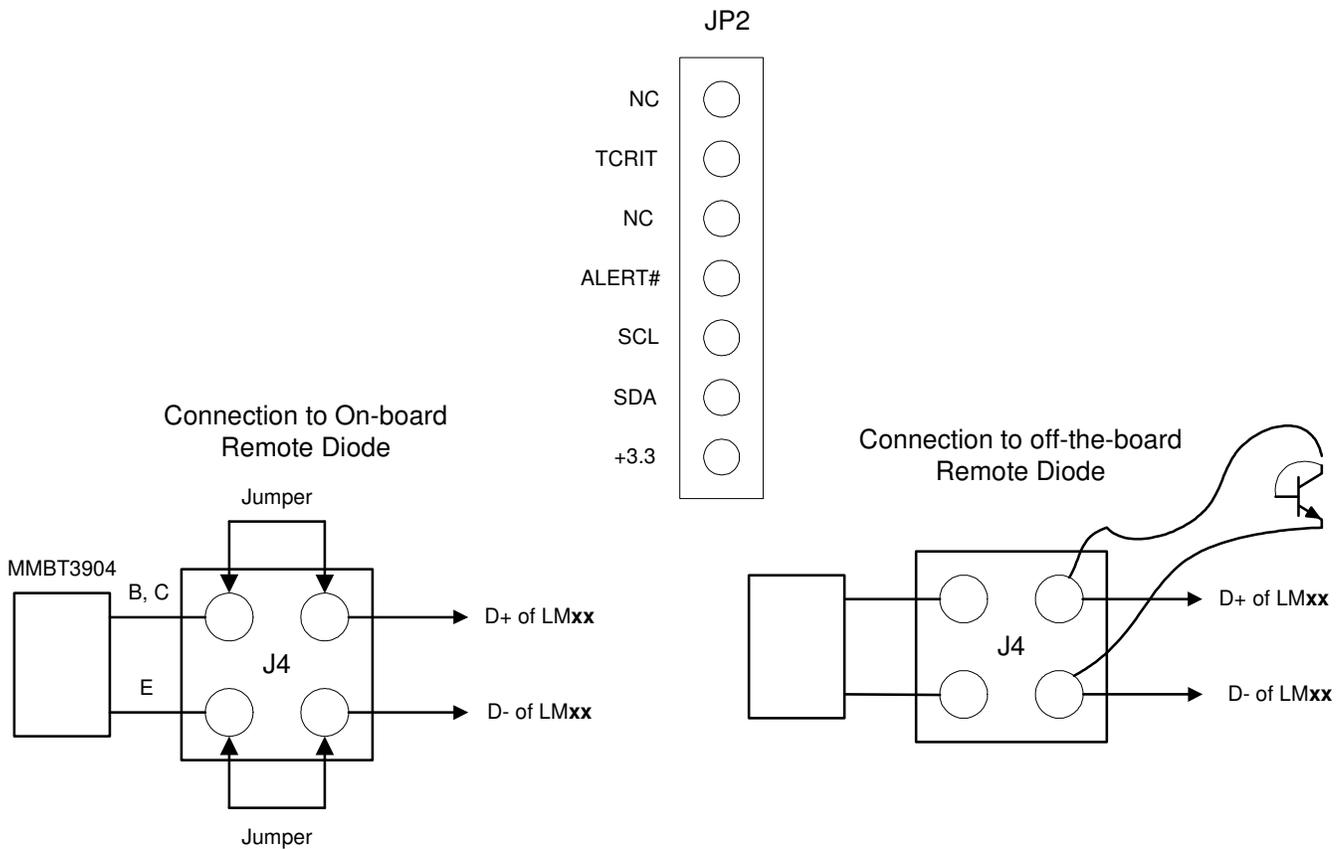
Figure 3. Header Connectors on the LMxx Evaluation Board
