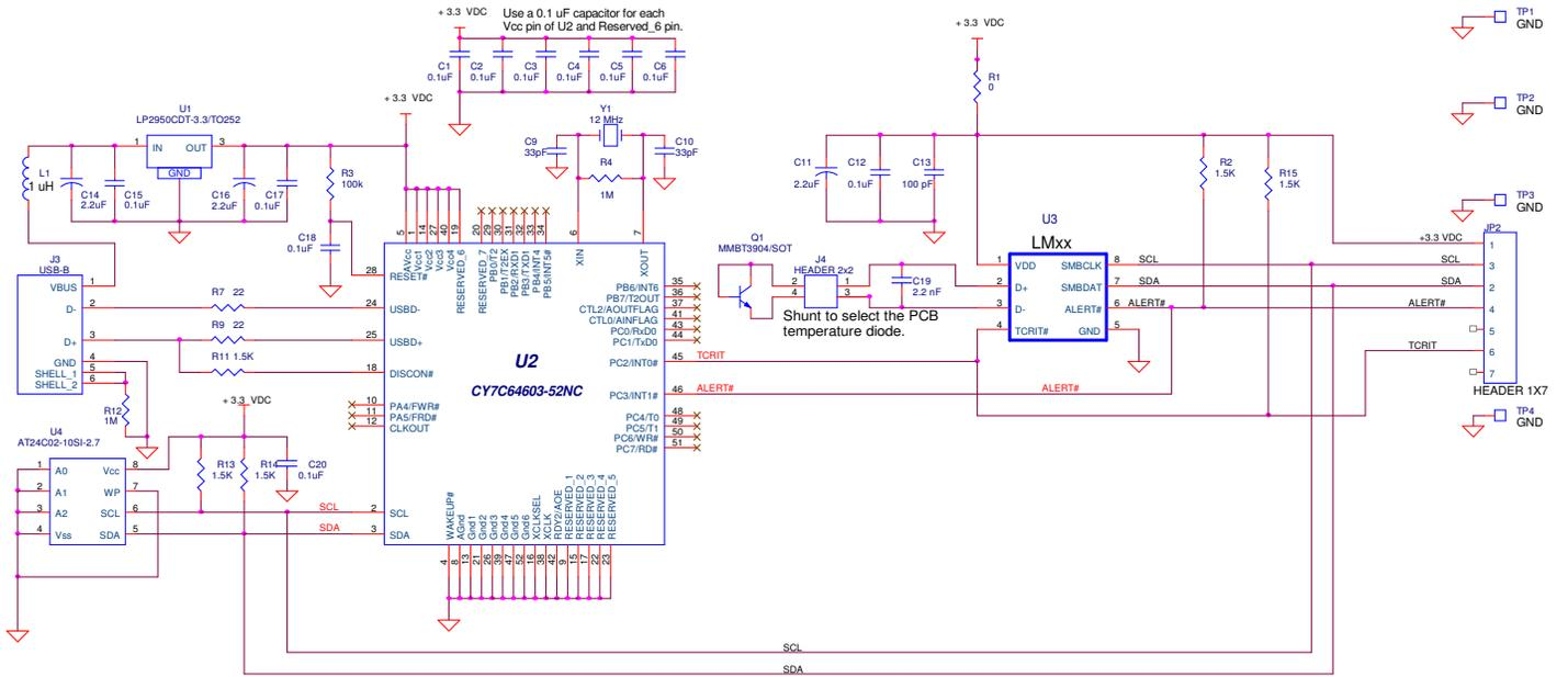
Figure 4. LMxx Evaluation Board Schematic
