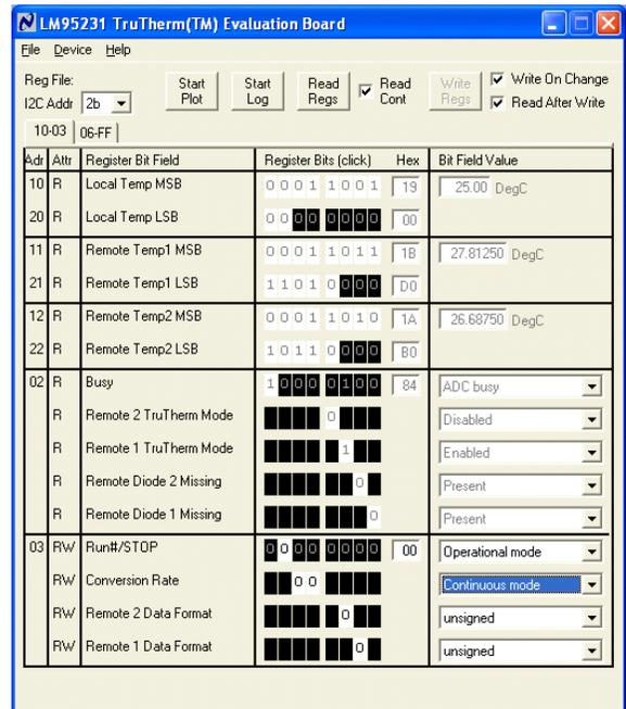
Local (on-chip), remote 1 (Q1 and Q2), and remote 2 (Q3), temperatures should read continuously.
