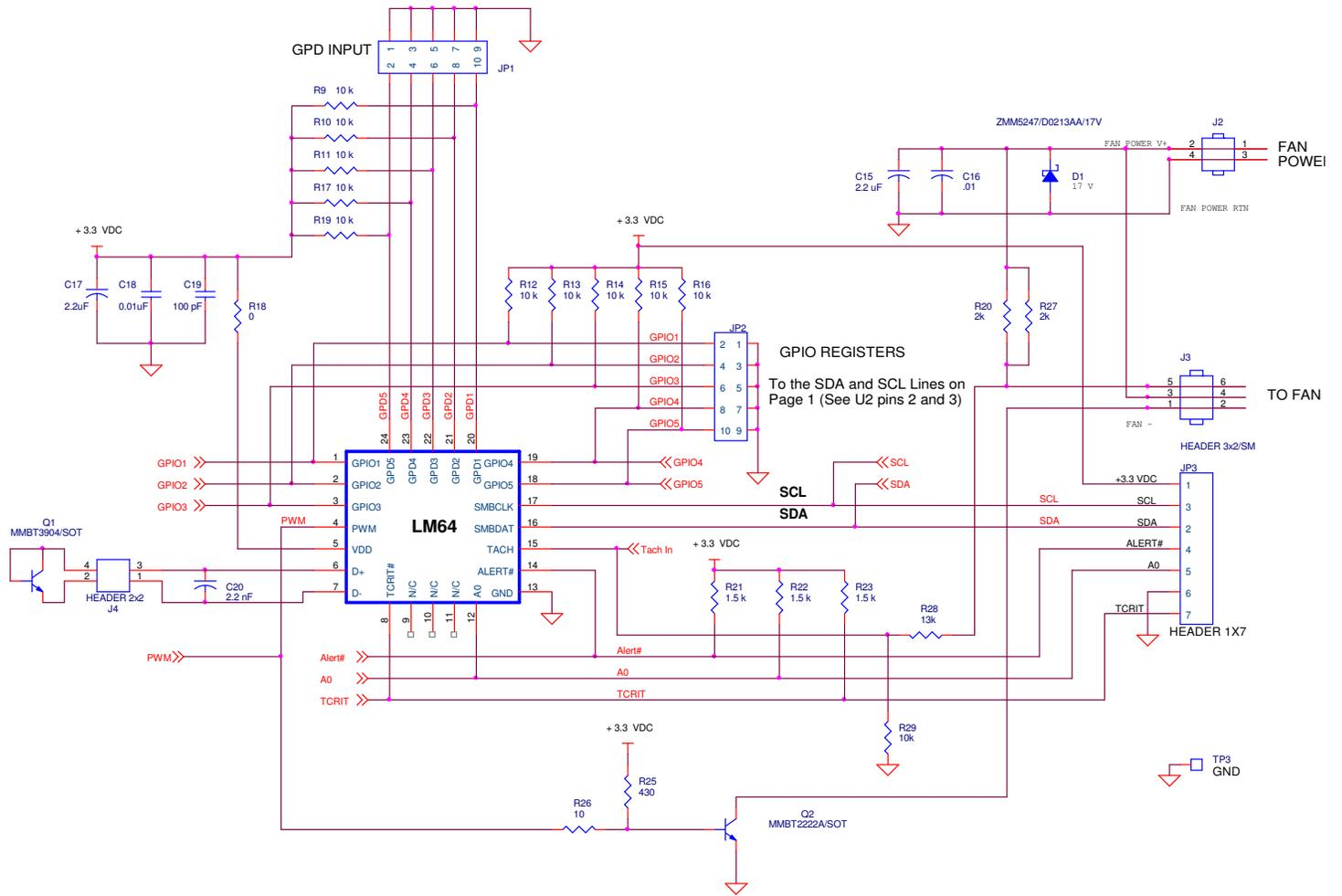
Figure 5b. Schematic of LM64 Evaluation Board – Page 2 of 2
