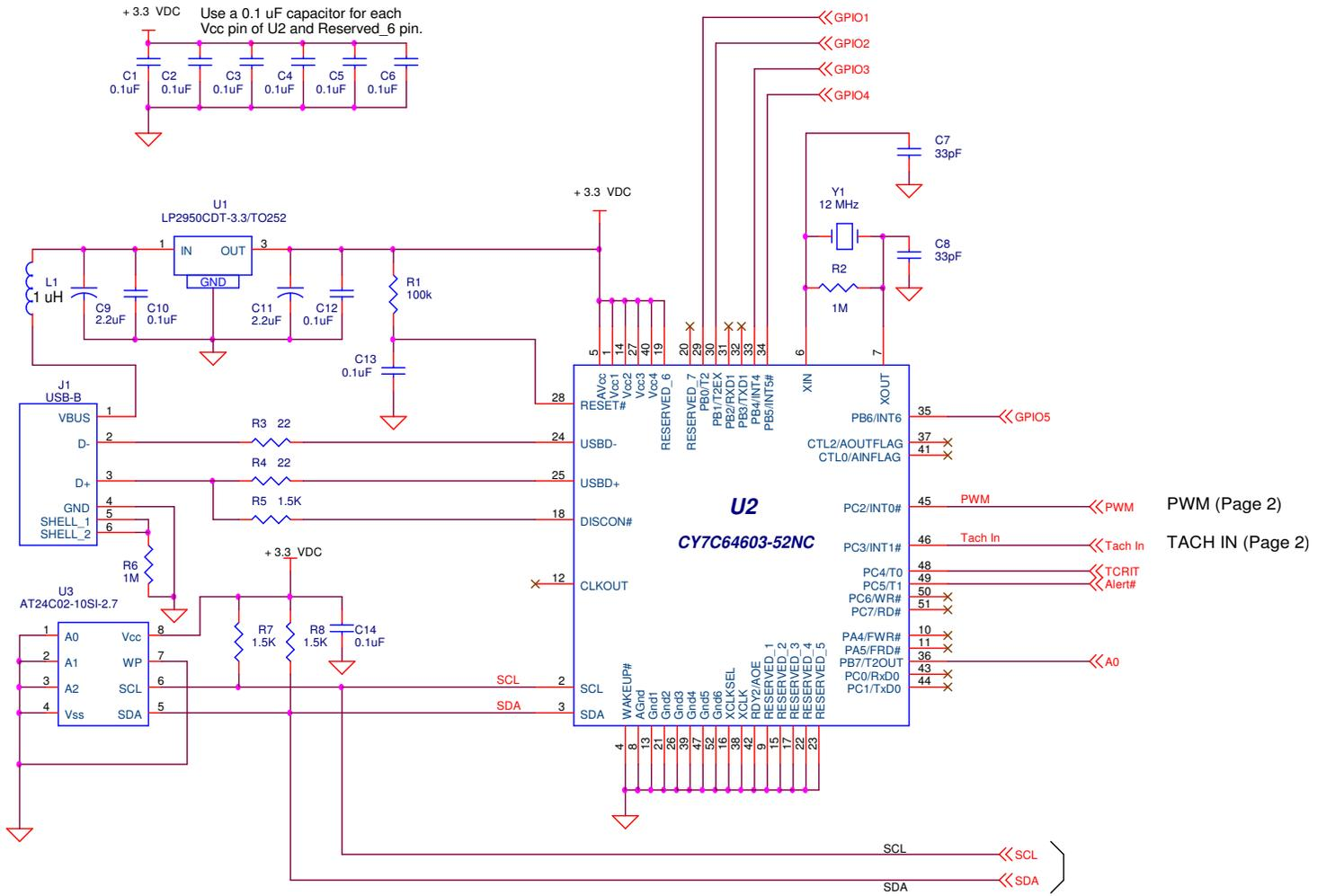
Figure 5a. LM64 Evaluation Board Schematic, Page 1 of 2
