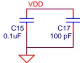
Use a 100 pF capacitor for each +3.3 V pin of U4, and U4S. Place 100 pF closest to the pin.
