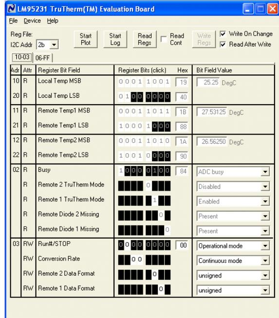
Select "Read Cont" to read the temperature continuously.
