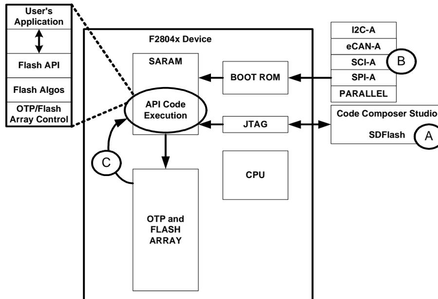
Method A: The code is loaded directly into on-chip SARAM via the JTAG port. This is the method used by Code Composer Studio and the SDFlash utility.
