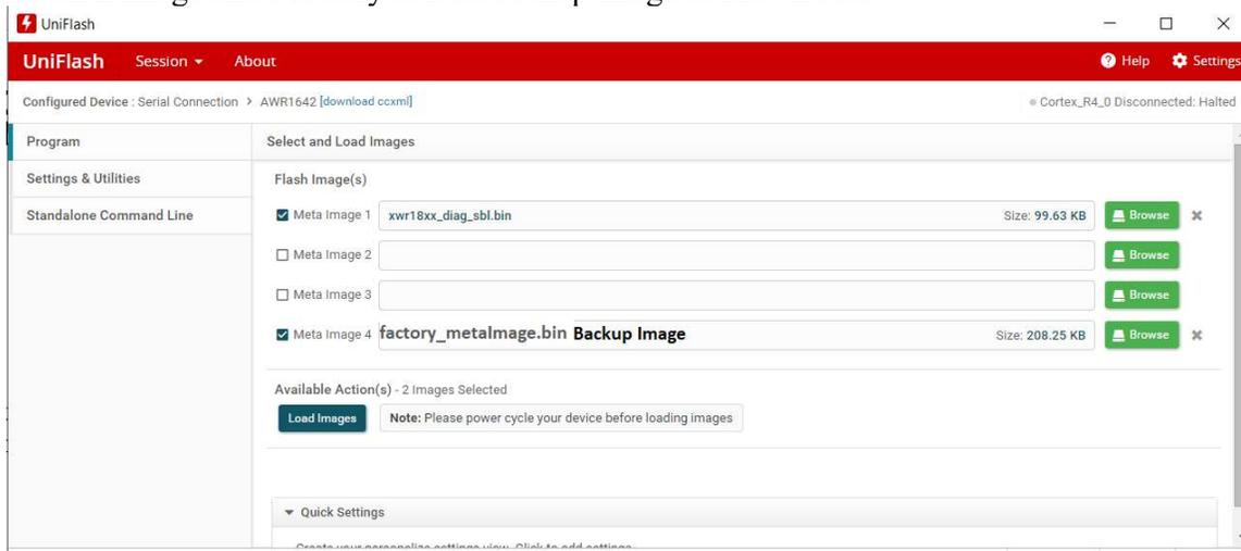
2. Find the COM port which shows as “XDS110 Class Application/User UART” under device manager. That COM no. needs to be set in ‘Setting & Utilities’ option of UniFlash.
