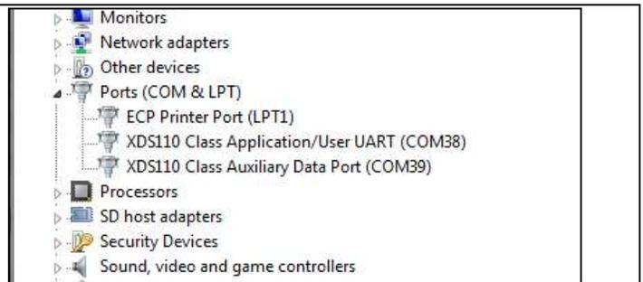
1. Connect to the COM port found in previous step (using any serial terminal application like Teraterm, Hyperterminal etc.) and configure the port (@baudrate 115200).
