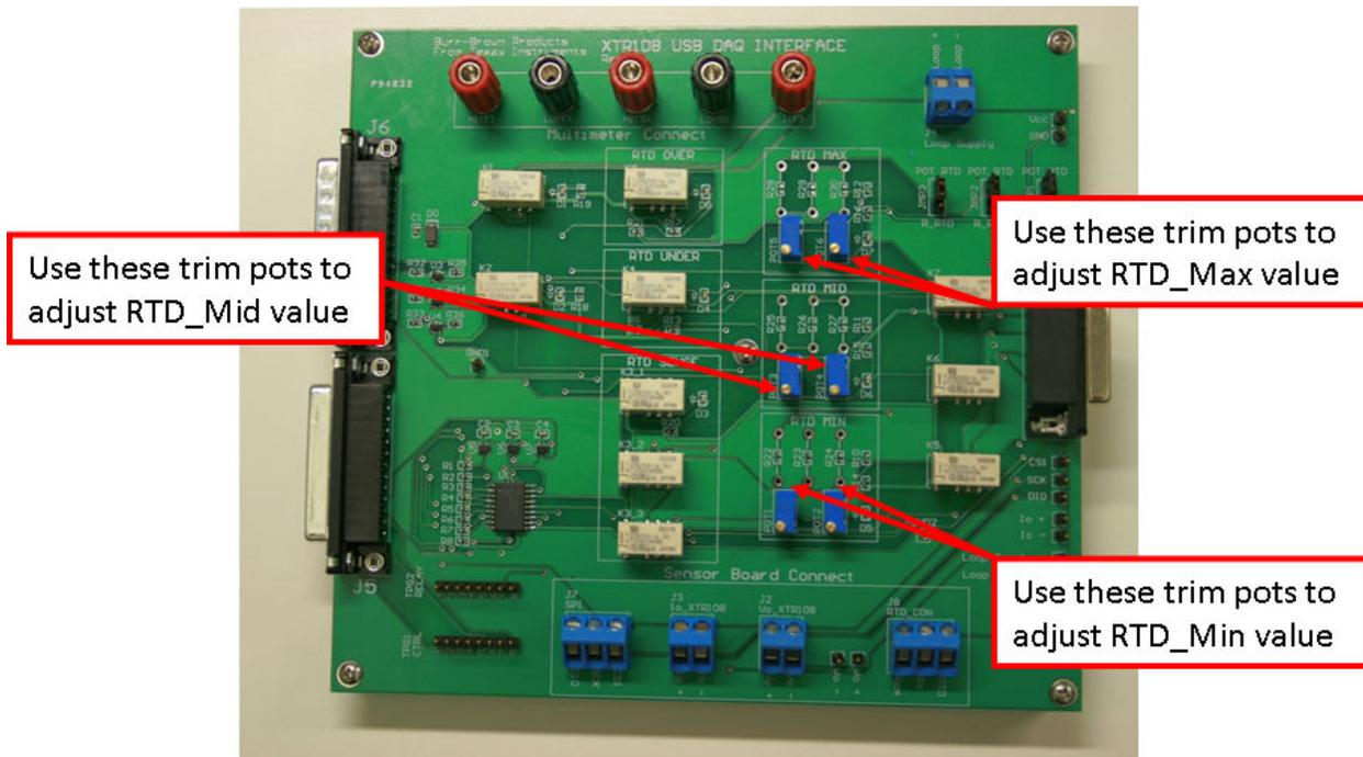
Make sure that your digital multi-meter is configured for four-wire resistance ( $\Omega$  4W) measurement in order to properly measure the RTD Emulator settings.
