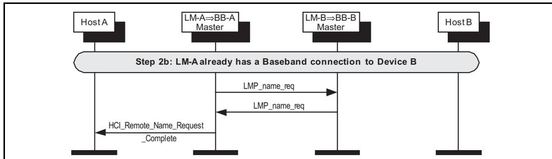
Figure 2.3: Remote name request with baseband connection.
