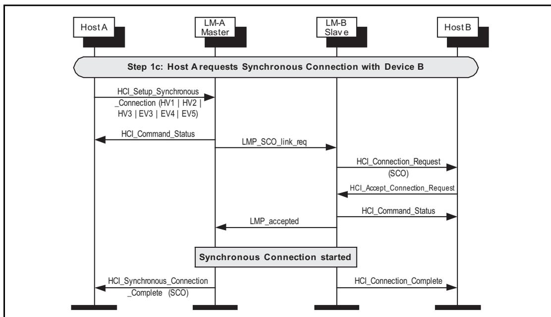
Figure 5.3: Master requests synchronous connection using SCO.
