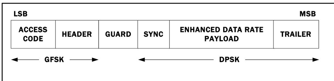
Figure 6.2: General enhanced data rate packet format
