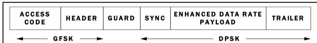
Figure 1.3: Standard Enhanced Data Rate packet format
