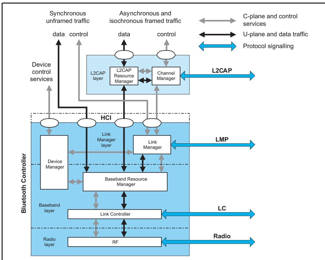
Figure 2.1: Bluetooth core system architecture
