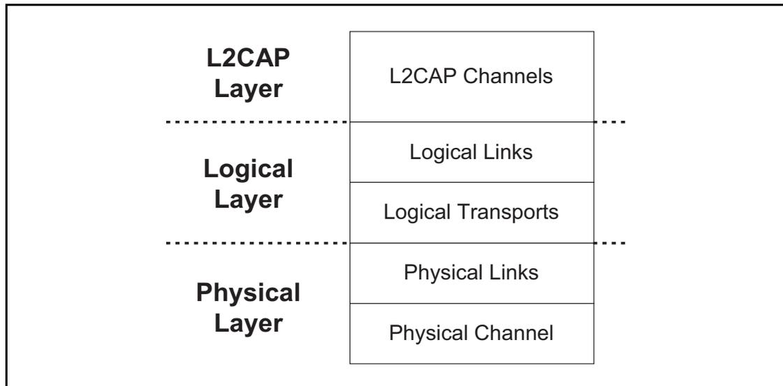
Figure 3.1: Bluetooth generic data transport architecture
