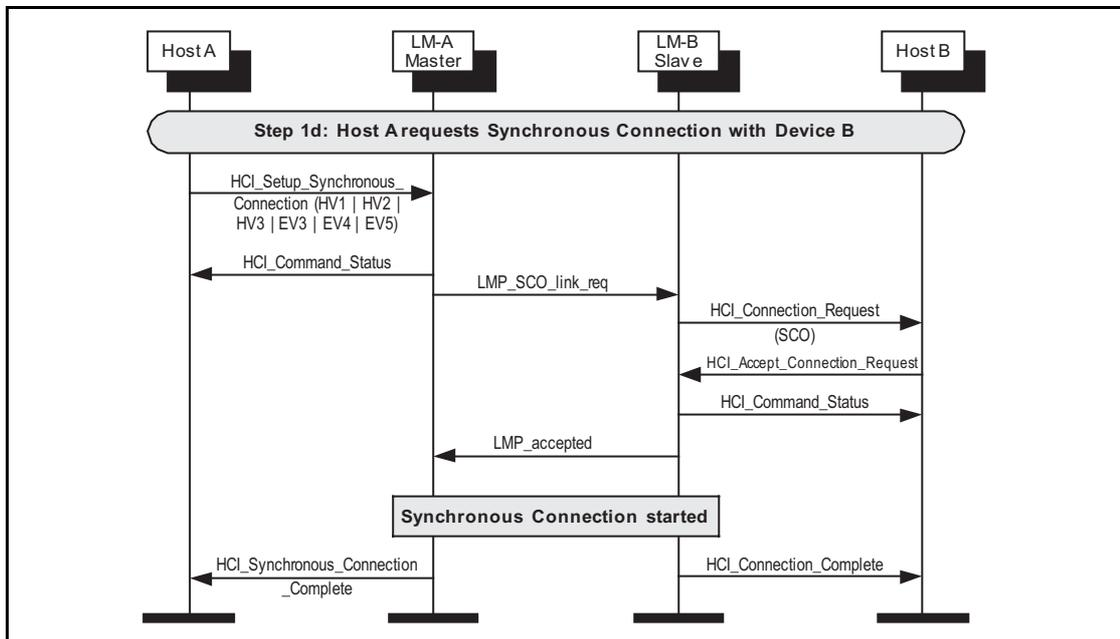
Figure 5.4: Master requests synchronous connection with legacy slave.
