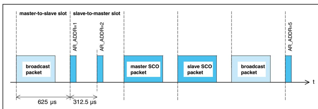
Figure 8.16: Disturbance of access window by SCO traffic
