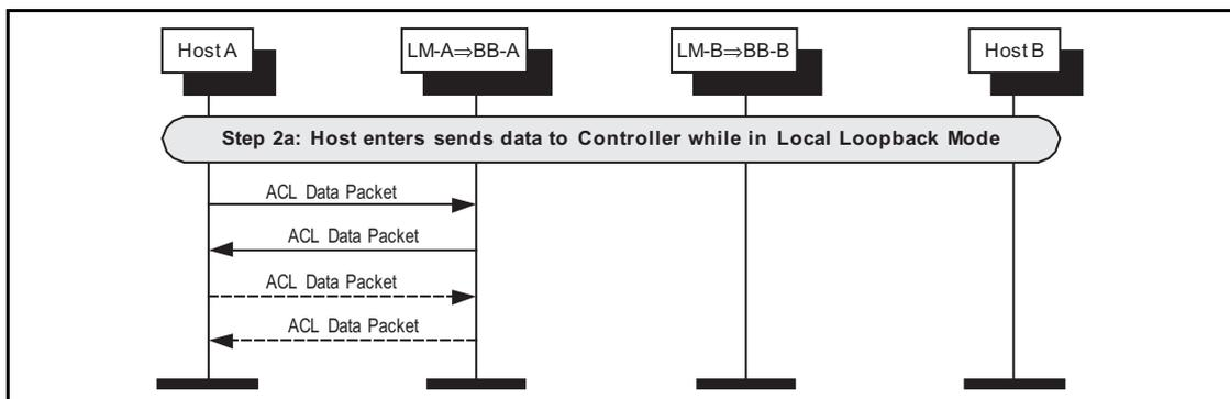
Figure 8.2: Looping back data in local loopback mode.
