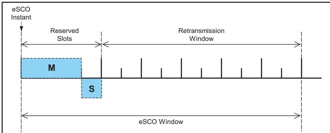
Figure 8.8: eSCO Window Details for Asymmetric Traffic
