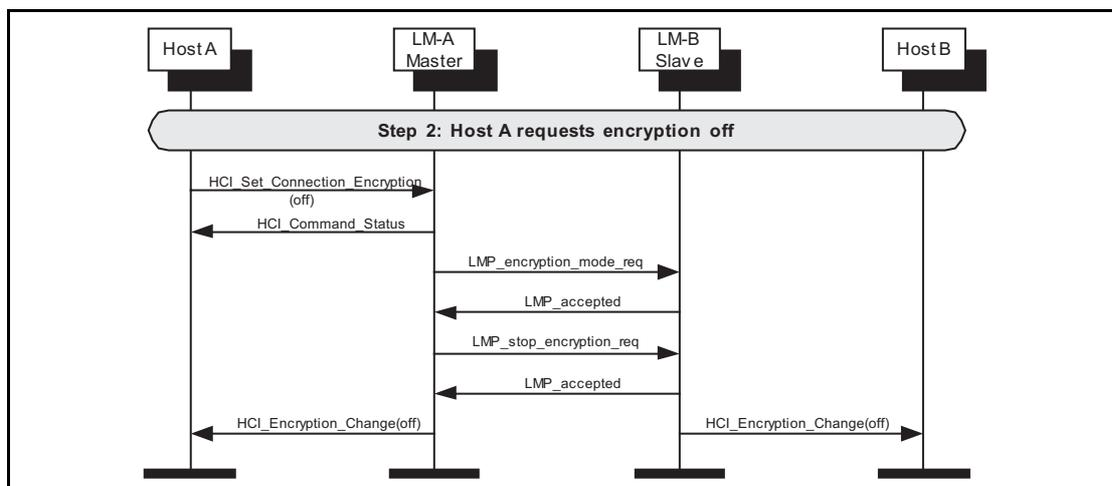
Figure 4.3: Encryption off requested.
