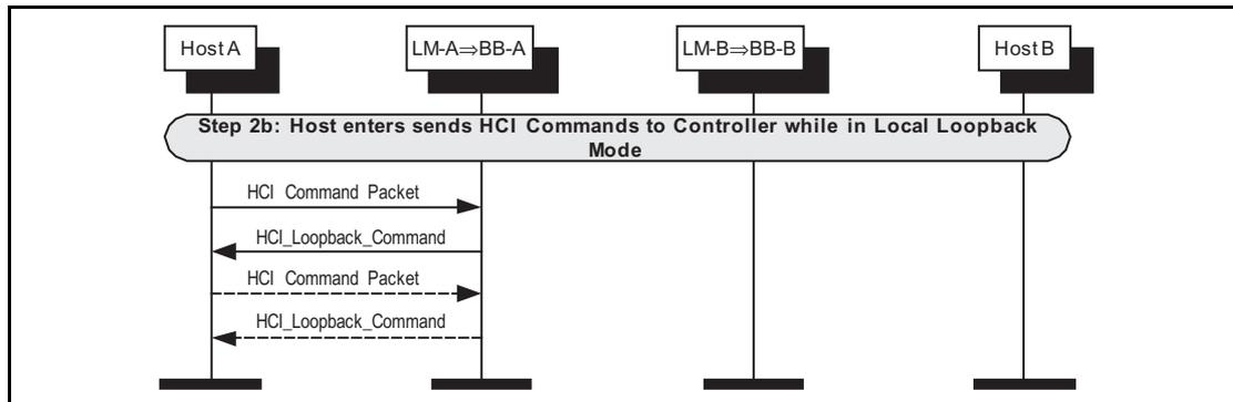
Figure 8.3: Looping back commands in local loopback mode.
