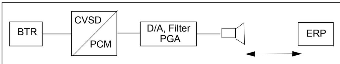
Figure 12.2: RLR measurement set-up.
