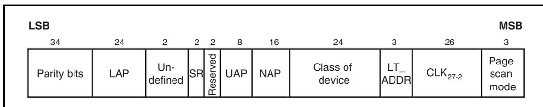
Figure 6.9: Format of the FHS payload.
