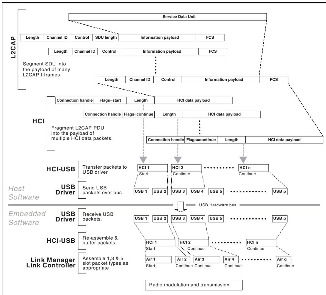
Figure 7.4: Example of segmentation and fragment processes in a device with HCI<sup>1</sup>
