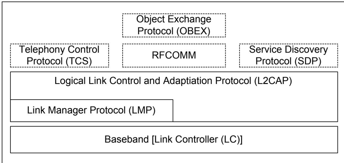
Figure 2.1: Profile stack covered by this profile.
