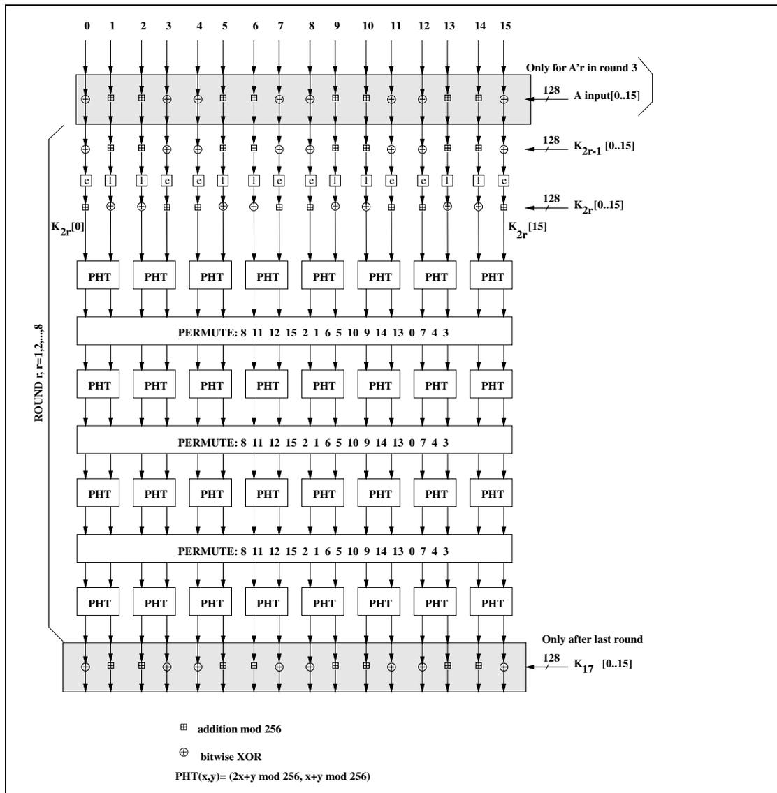
Figure 6.2: One round in  $A_r$  and  $A'_r$ . The permutation boxes show how input byte indices are mapped onto output byte indices. Thus, position 8 is mapped on position 0 (leftmost), position 11 is mapped on position 1, etc.
