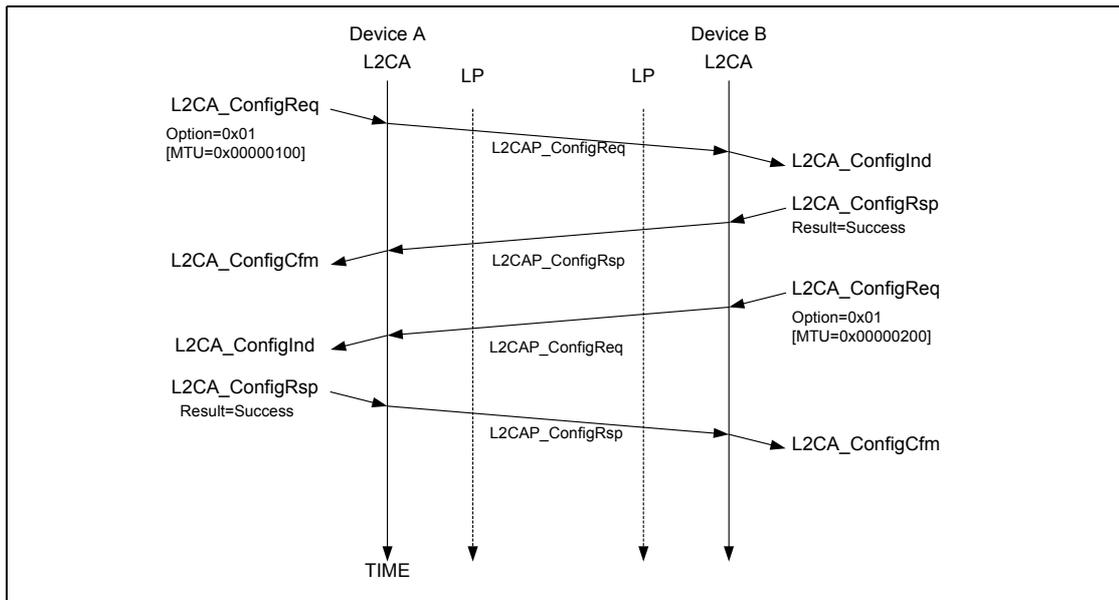
Figure I: Basic MTU exchange
