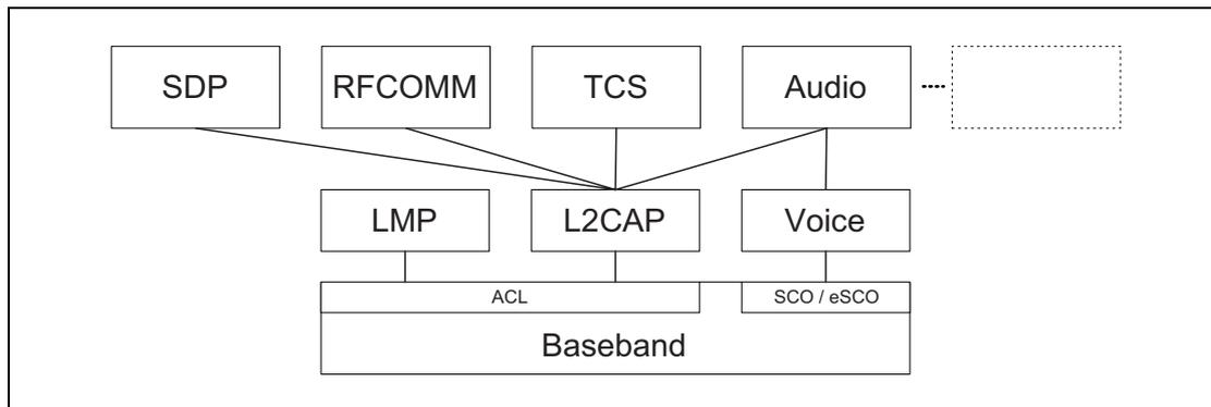
Figure 1.2: L2CAP data flows in Bluetooth Protocol Architecture
