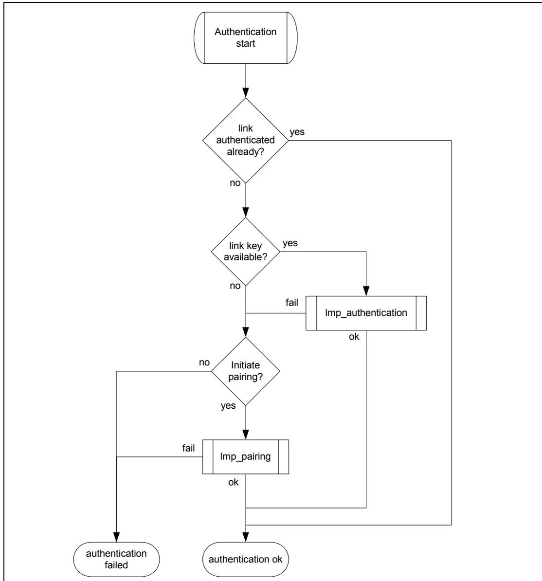
Figure 5.1: Definition of the generic authentication procedure.
