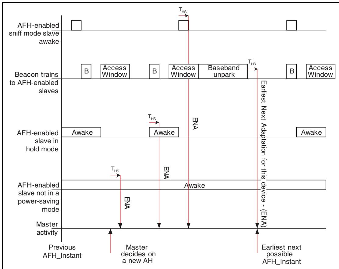
Figure 12.4: Timing constraint on AFH\_Instant with slaves in park, hold and sniff
