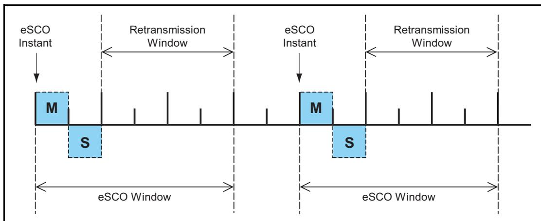
Figure 8.7: eSCO Window Details for Single-Slot Packets
