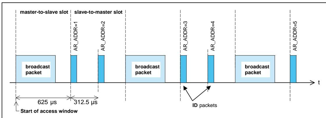
Figure 8.15: Access procedure applying the polling technique.
