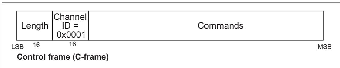
Figure 4.1: L2CAP PDU format on the signalling channel
