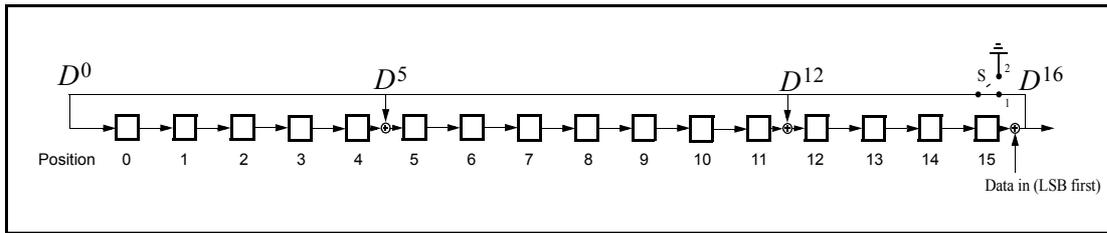
Figure 7.6: The LFSR circuit generating the CRC.
