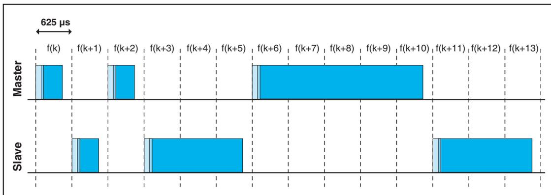
Figure 2.1: Multi-slot packets
