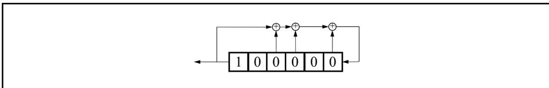
Figure 6.6: LFSR and the starting state to generate  $p'(D)$ .
