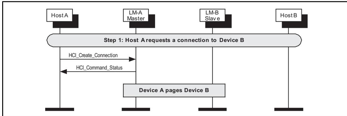
Figure 3.2: Host A requests connection with device B.
