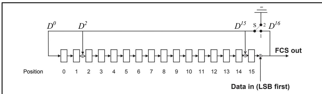
Figure 3.4: The LFSR circuit generating the FCS.
