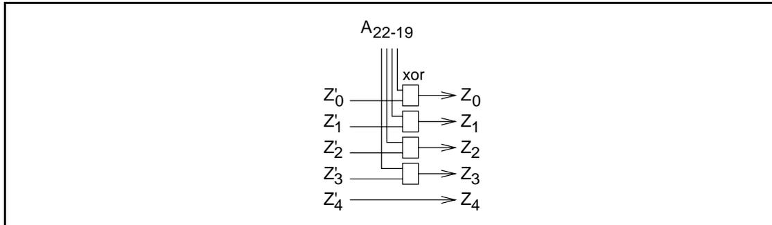
Figure 2.17: XOR operation for the hop system.
