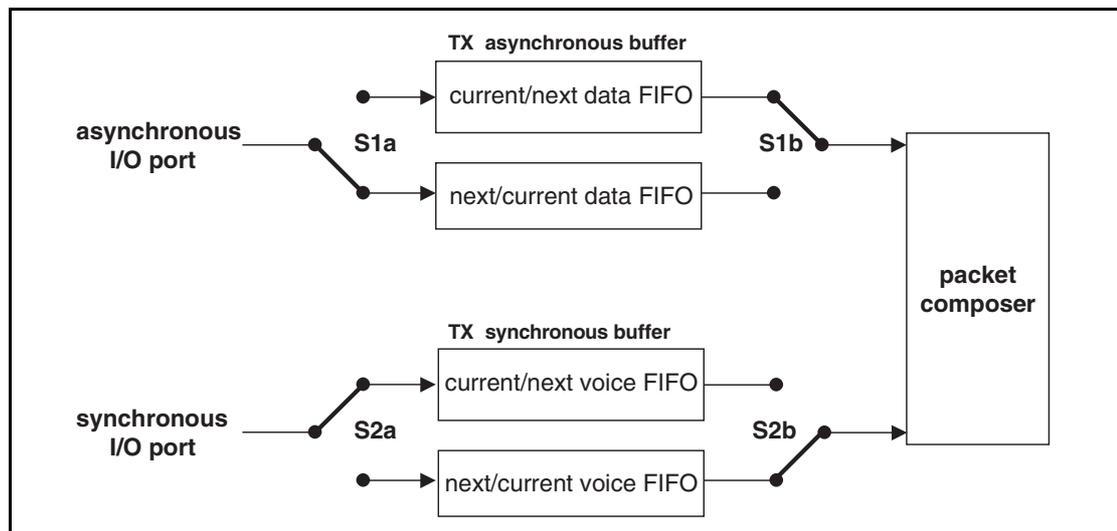
Figure 4.1: Functional diagram of TX buffering.
