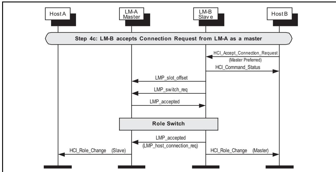
Figure 3.7: Device B accepts connection requests as master.
