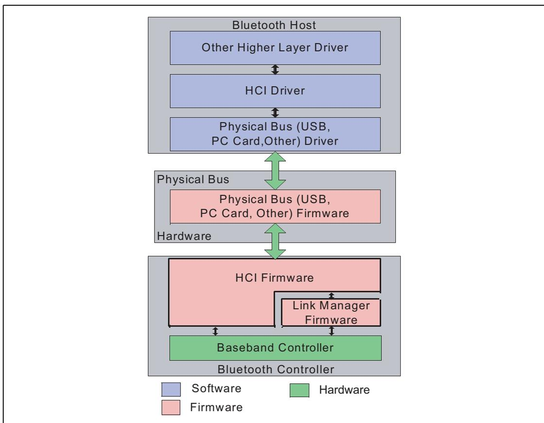
Figure 1.1: Overview of the Lower Software Layers
