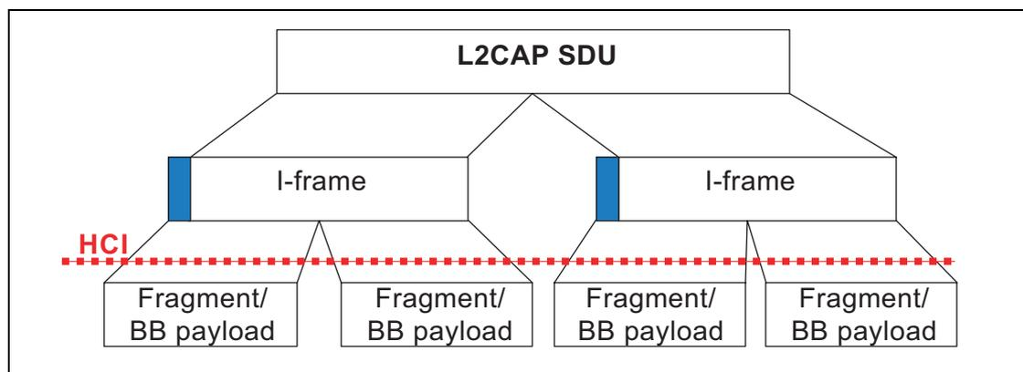
Figure 7.3: Segmentation and fragmentation of an SDU.
