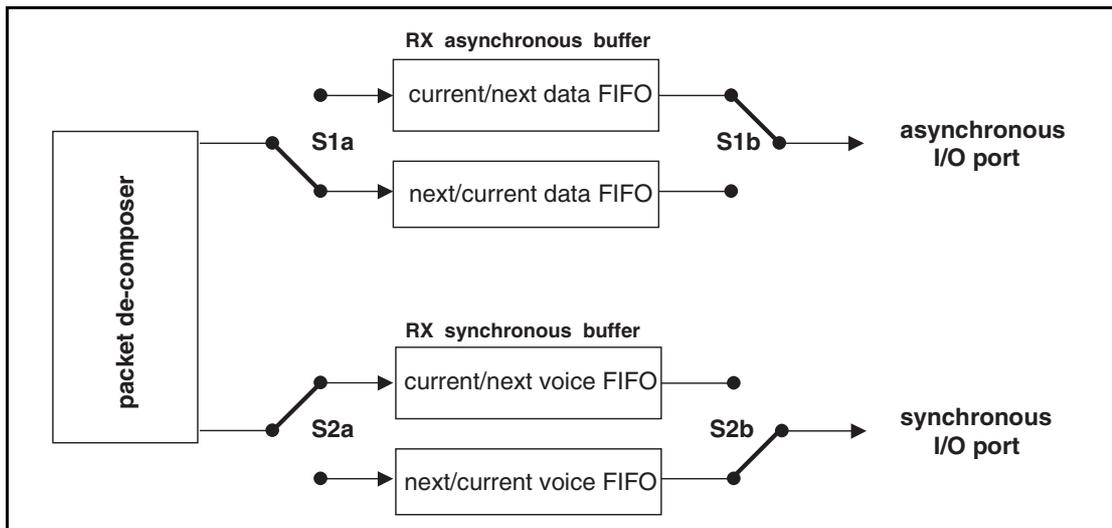
Figure 4.2: Functional diagram of RX buffering
