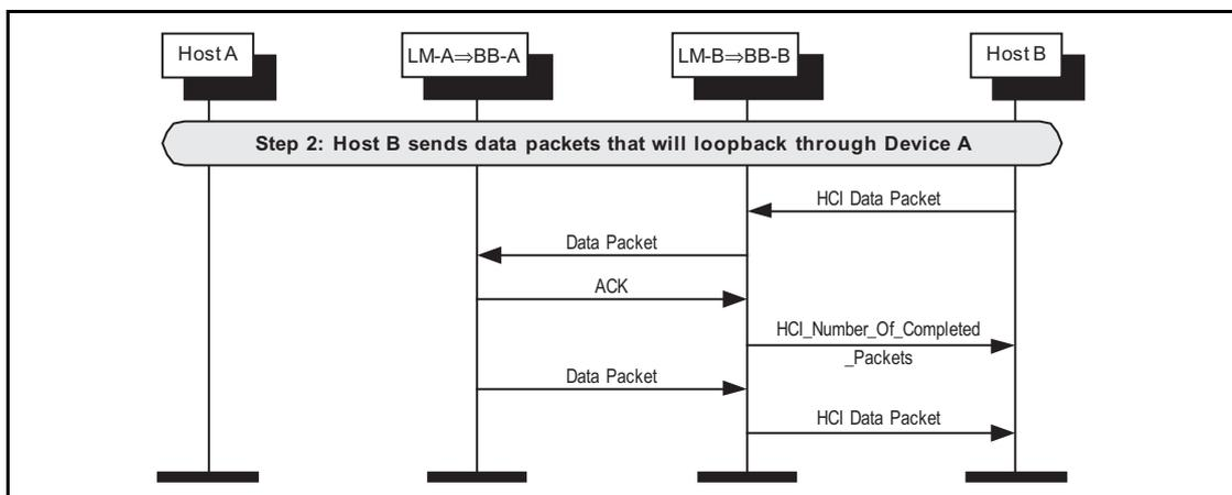
Figure 8.6: Looping back data in Remote Loopback Mode.
