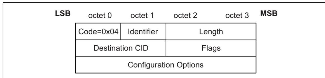
Figure 4.6: Configuration Request Packet
