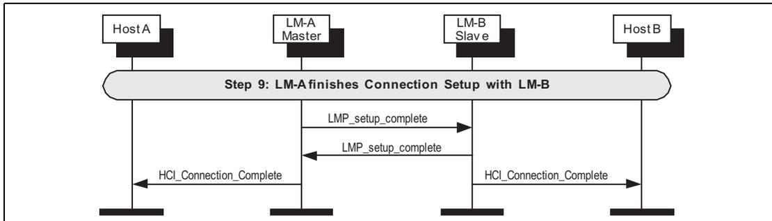
Figure 3.13: LM-A and LM-B finishes connection setup.
