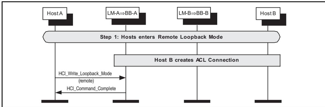
Figure 8.5: Entering remote loopback mode.
