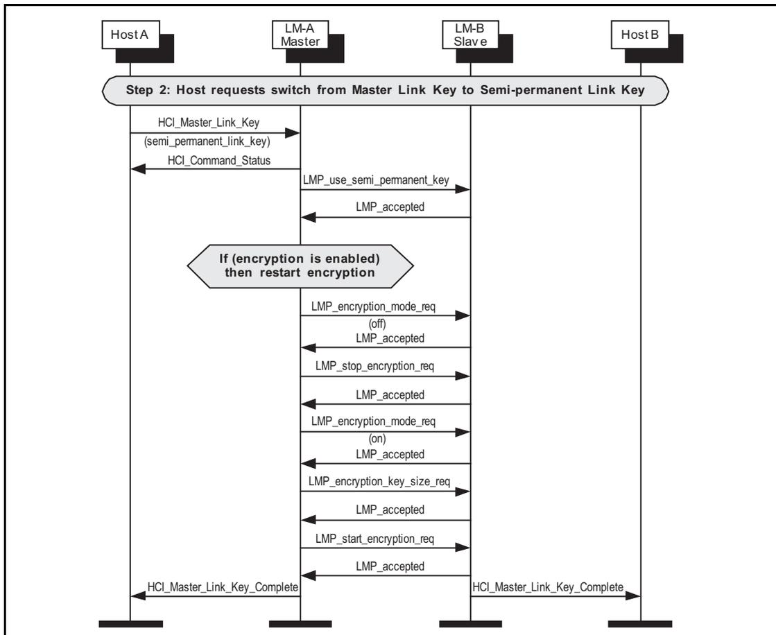
Figure 4.6: Change to semi permanent link key.
