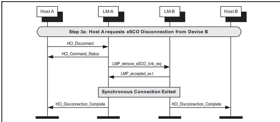
Figure 5.8: Synchronous disconnection of eSCO connection.
