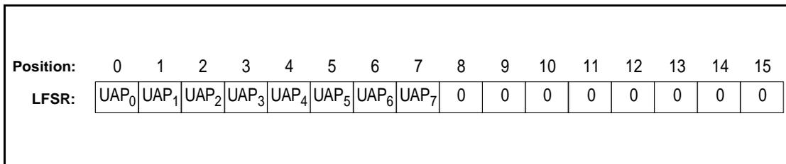
Figure 7.7: Initial state of the CRC generating circuit.
