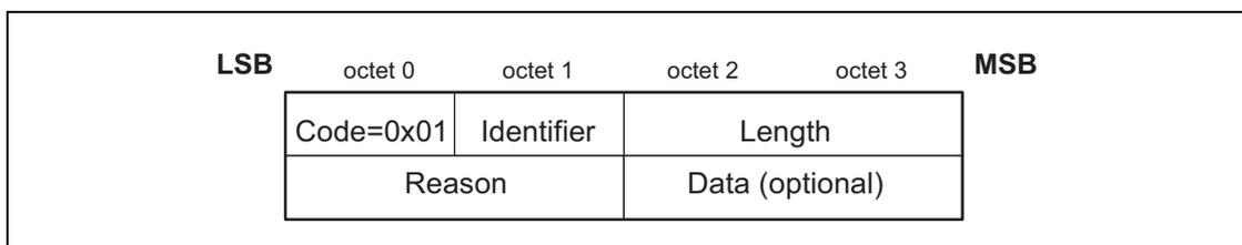
Figure 4.3: Command Reject packet
