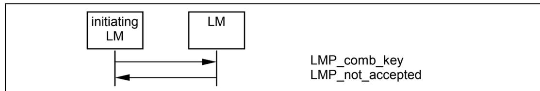
Sequence 30: Change of the link key not possible since the other device uses a unit key.
