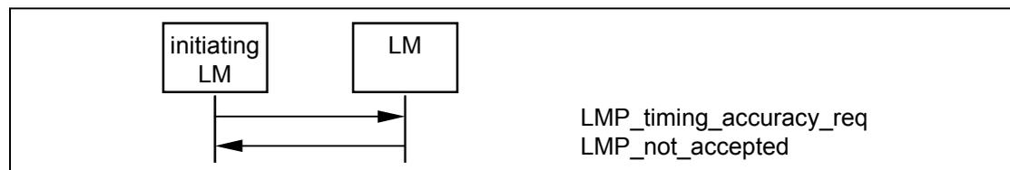
Sequence 40: The requested device does not support timing accuracy information.
