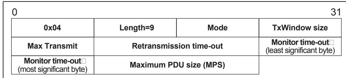
Figure 5.5: Retransmission and Flow Control option format.
