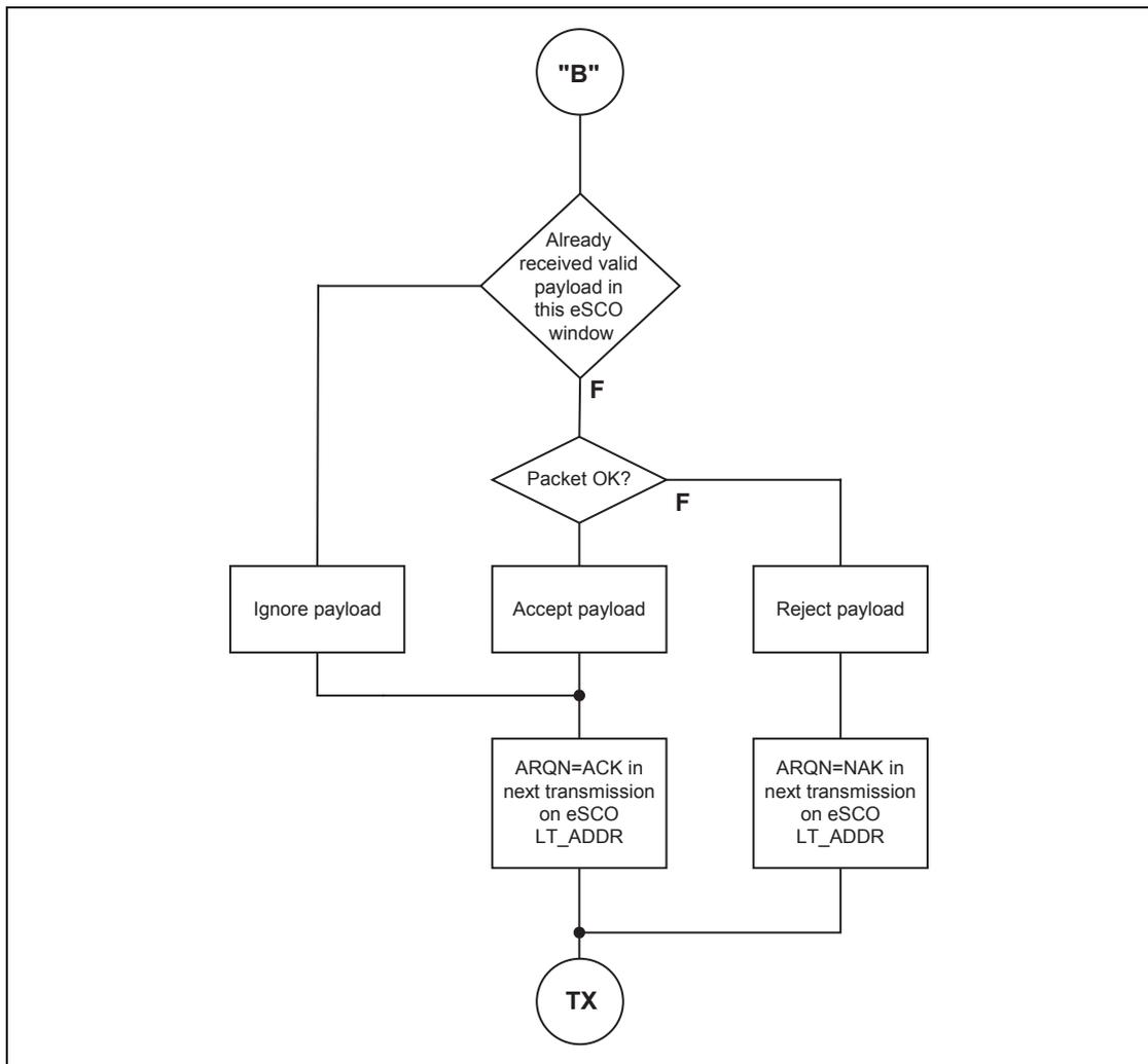
Figure 7.14: Stage 2 (eSCO) of the receive protocol for determining the ARQN bit.
