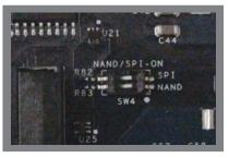
Configure switch SW4: NAND=OFF, SPI=OFF.
