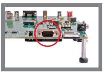
Connect supplied serial cable to UART (P10). Connect the other end of the serial cable to a PC. This step is not required for initial EVM start-up, it is optional. This step enables viewing of console messages on a PC terminal and changing some of the default parameters on the EVM.
