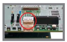
Connect the supplied USB mouse to the top connector of the USB port (J13).
