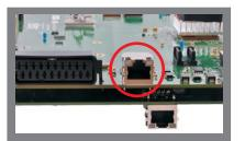
Connect the supplied Ethernet cable to the RJ-45 jack on the board (J10). Connect the other end of the cable to an Internet-ready connection (router/switch). This step is not required for initial EVM start-up, it is optional. This step allows proper execution of example applications that use Internet access.
