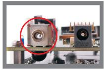
Turn power switch (SW1) to the ON position (closest position to the corner of the PCB board).
