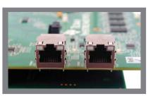
Connect the supplied Ethernet cable to the RJ-45 jack on the board (J14 or J27). Connect the other end of the cable to an Internet-ready connection (router/switch). This step is not required for initial EVM startup, it is optional. This step allows proper execution of example applications that use Internet access.
