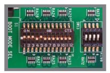
For SD boot set up, configure S1 switches 1, 2, 3, 5 = ON; all other switches OFF.
