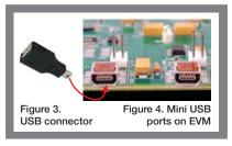
Connect the supplied USB adaptor (Figure 3) to the mouse. Then connect the mini side of the adaptor to the USB port (Figure 4) MI (J2 or J3).
