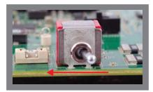
Turn power switch (SW1) in the direction of the arrow shown.
