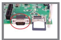
Connect supplied serial cable to UART (P2). Connect the other end of the serial cable to a PC. This step is not required for initial EVM start-up, it is optional. This step enables viewing of console messages on a PC terminal and changing some of the default parameters on the EVM.
