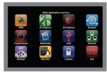
Application Launcher should display on the LCD within approximately one minute. Note: By default, the HDMI output is set to 1080p. To change output resolution, please refer to the Software Development Guide (provided in the SDK installer on the SD card). (Please note: Application Launcher icons on LCD may vary from picture shown here. This is shown for reference only.)
