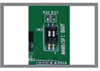
Configure SW2 switches (for NAND and SPI) as OFF.
