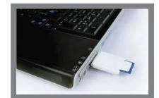
When you are ready to start programming the DM814x/AM387x EVM, please remove power to the board, remove the Linux™ SDK SD card and insert into the included and unplugged USB SD card reader. On a Linux host PC running the Ubuntu 10.04 distribution, insert the reader into any unused USB port and from the START HERE folder, run setup.htm.
