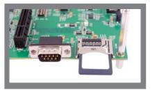
Insert the supplied SD card into the SD card slot, with SD card label facing up (J15).
