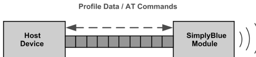
Profile Data Sent/Received To/From the SB module
