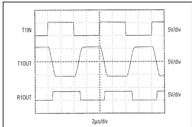
Figure 11. MAX3224E/MAX3226E/MAX3244E Loopback Test Result at 250kbps
