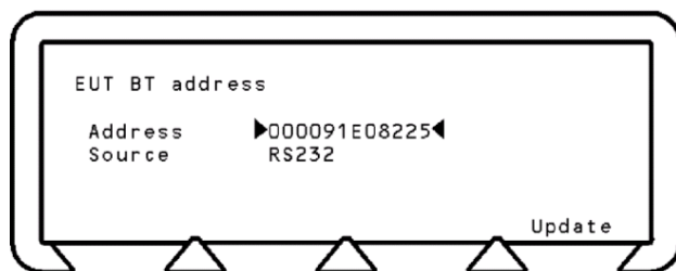
Figure 2. BD_ADDR Captured by an Anritsu MT8852A Bluetooth Test Set
