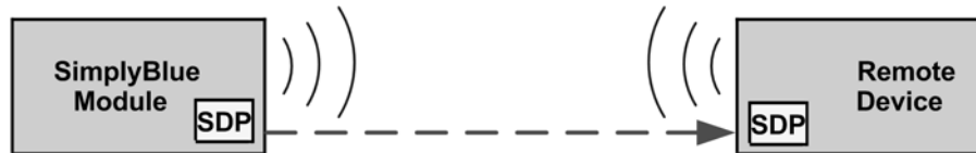
SB device initiates the SPP link establishment
