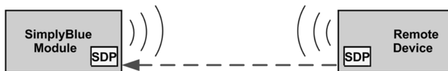
Remote device initiates the SPP link establishment
