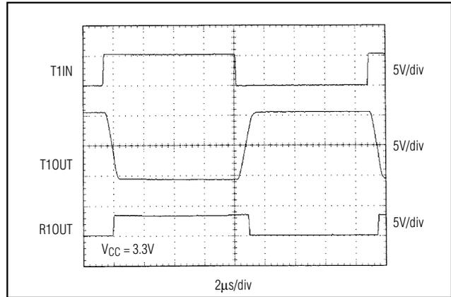
Figure 10. MAX3224E/MAX3226E/MAX3244E Loopback Test Result at 120kbps
