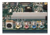
**4.** Connect your 720P capable HD video display to the component video out RCA connector. Power on the HD video display.
