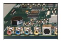
**5.** Connect an audio speaker to stereo line out and an audio source to stereo line in.
