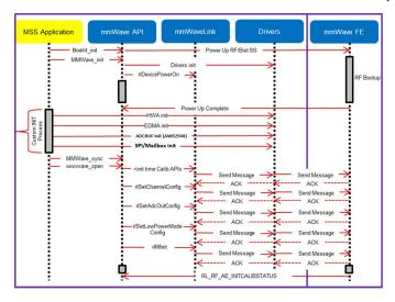
5.3.1.2.1. Figure 10: mmWave Isolation mode: Detailed Control Flow (Init sequence)
