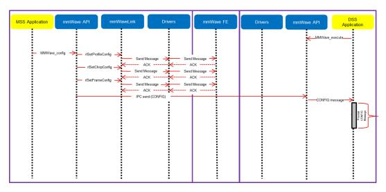
5.3.1.3.2. Figure 14: mmWave Co-operative Mode: Detailed Control Flow (Config sequence)
