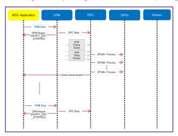
5.3.2.2.2. Figure 18: Data processing flow with local domain control (start/chirp/frame/stop)
