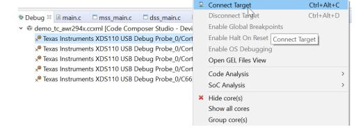
8. After connecting to either Cortex\_R5\_0 or C66xx\_DSP core, **perform a CPU Reset** on each of the cores by selecting them one by one and clicking on "CPU Reset".
