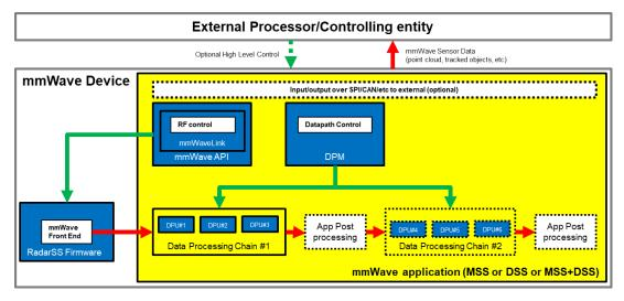
5.1.1.1.1. Figure 4: Autonomous mmWave sensor (Standalone mode)
