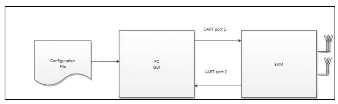
3.4.1.1 Figure 1: mmWave Demo Visualizer- mmWave Device Connectivity
