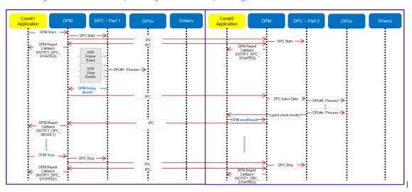
5.3.2.4.2. Figure 22: Distributed Data processing flow and control (start/chirp/frame/stop)
