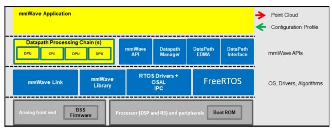
5.1.1.1.2. Figure 5: SDK Layered block diagram
