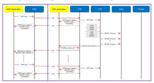
5.3.2.3.2. Figure 20: Data processing flow with remote domain control (start/chirp/frame/stop)
