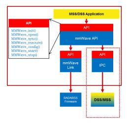
5.5.4.1.1. Figure 24: mmWave API - Internal software design
