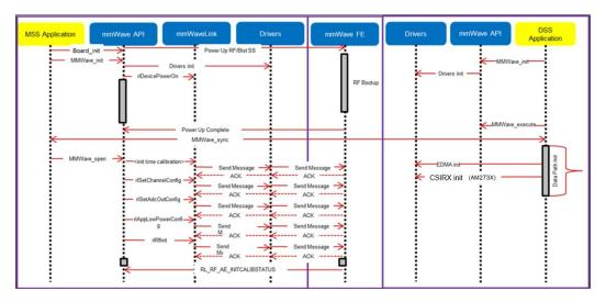
5.3.1.3.1. Figure 13: mmWave Co-operative Mode: Detailed Control Flow (Init sequence)
