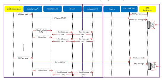
5.3.1.3.3. Figure 15: mmWave Co-operative Mode: Detailed Control Flow (Start sequence)
