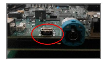
Connect a Debug USB via mini-USB connector. Connect
