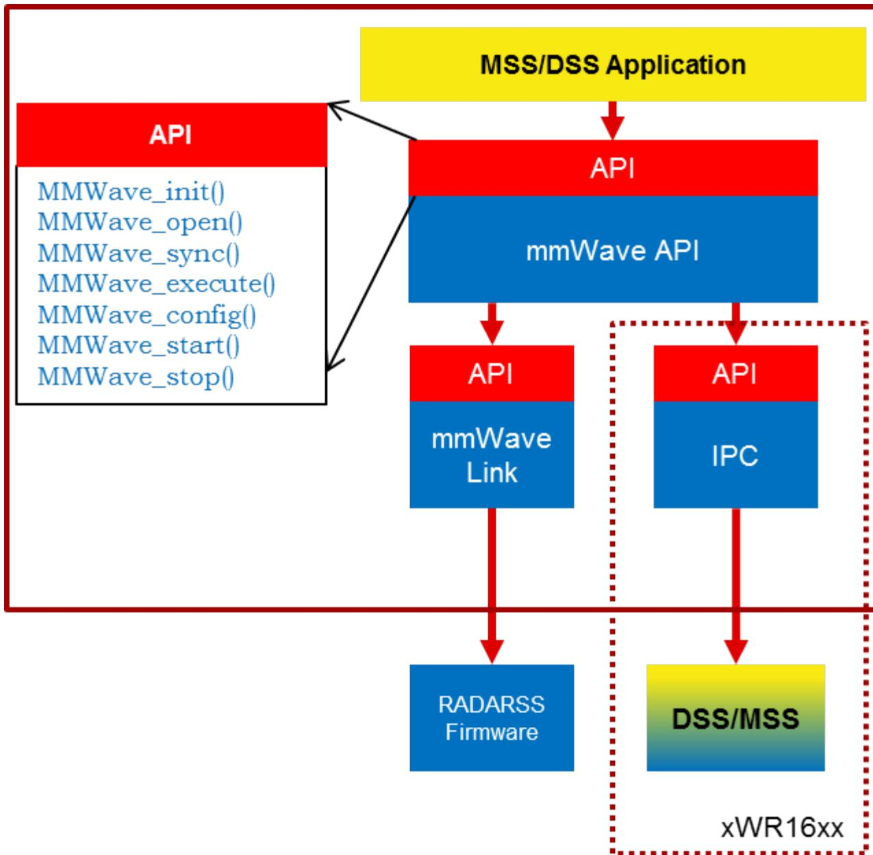
5.4.5.0.4Figure 27: mmWave API - Internal software design
