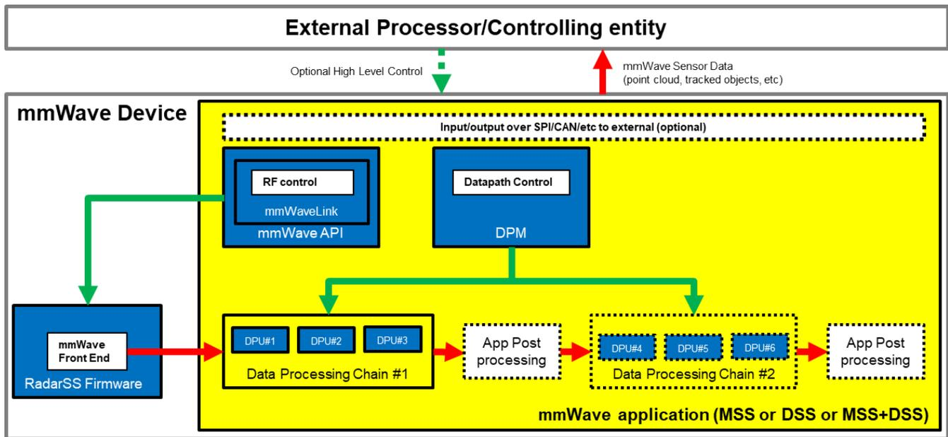
5. 1. 0. 0. 1Figure 6: Autonomous mmWave sensor (Standalone mode)
