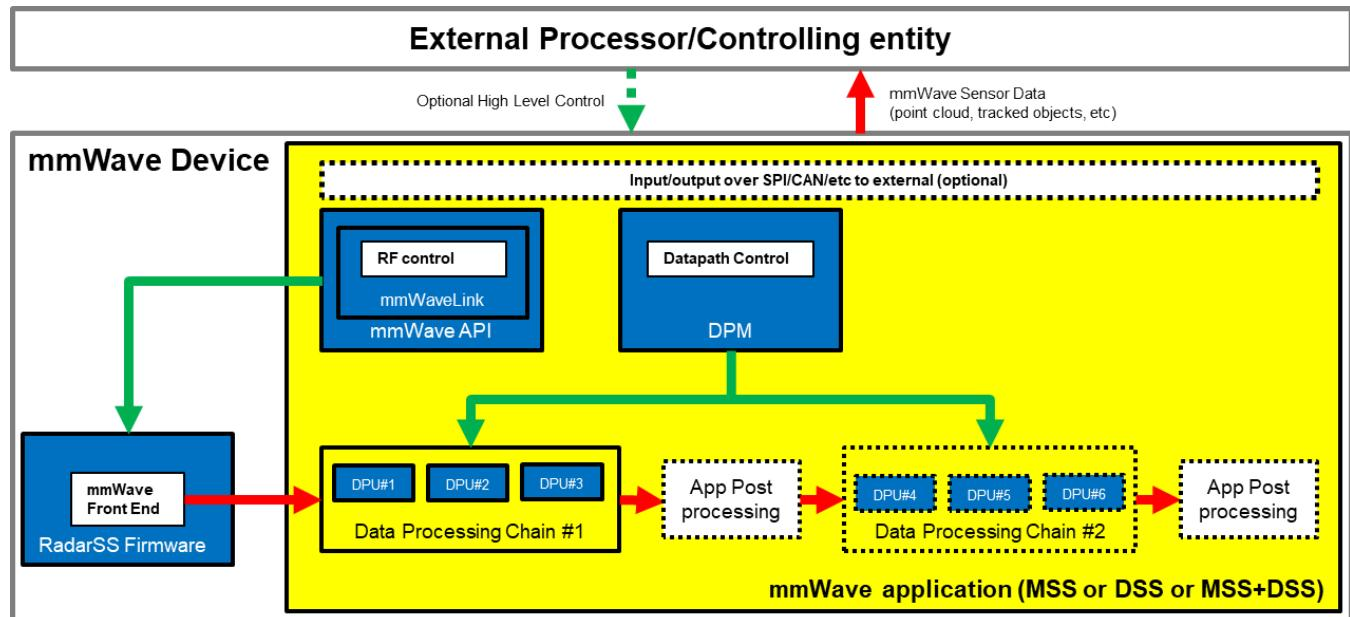
[5.1.0.0.1](#)Figure 6: Autonomous mmWave sensor (Standalone mode)
