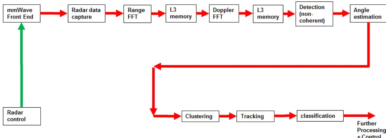
5. 2. 0. 0. 1Figure 8: Typical mmWave radar processing chain
