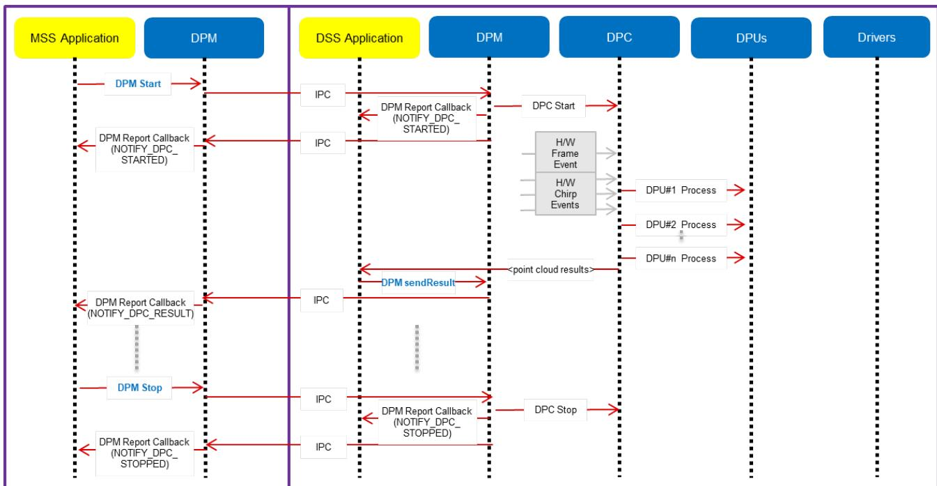
5.3.2.2 Figure 22: Data processing flow with remote domain control (start/chirp/frame/stop)
