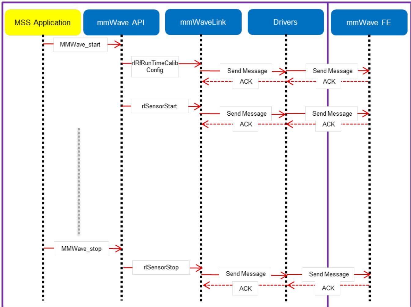
5. 3. 1. 3Figure 14: mmWave Isolation mode: Detailed Control Flow (start sequence)
