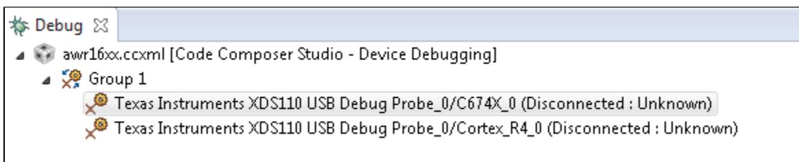
4.4.3.2.1Figure 5: Connecting to mmWave Device in CCS
