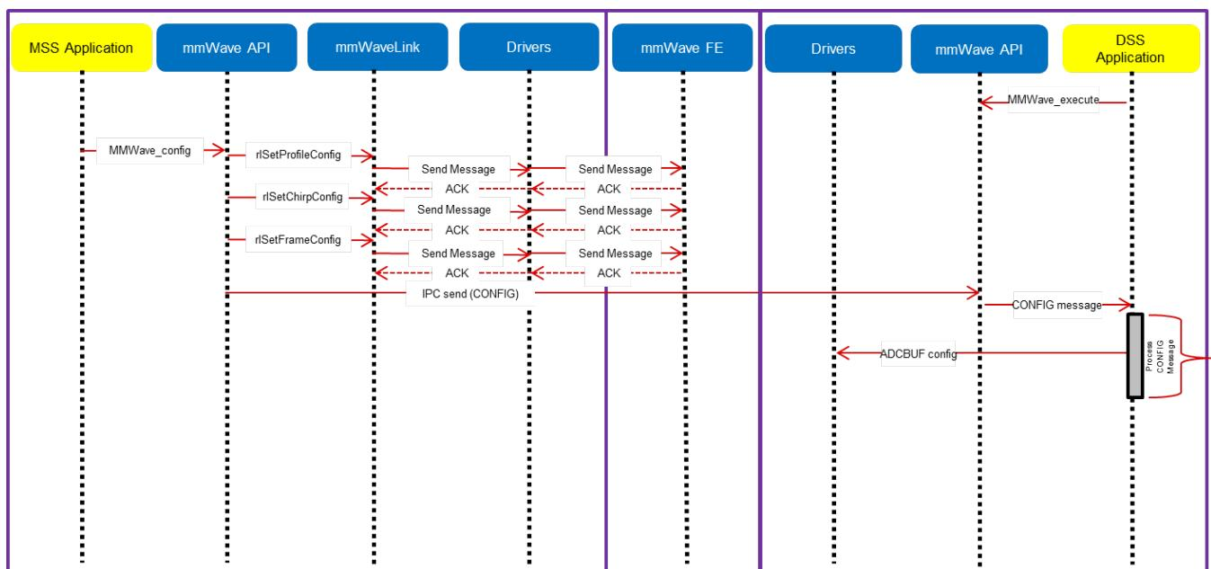
5. 3. 1. 2Figure 16: mmWave Co-operative Mode: Detailed Control Flow (Config sequence)
