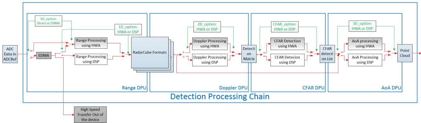
5.2.0.1Figure 10: Scalable data processing chain using mmWave SDK
