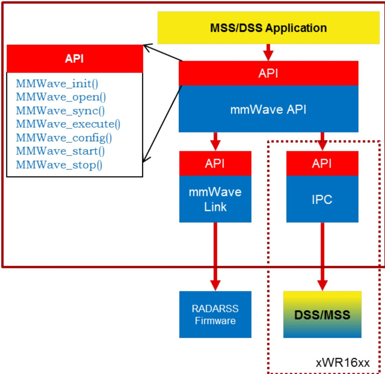
5. 4. 5. 0. 4Figure 27: mmWave API - Internal software design
