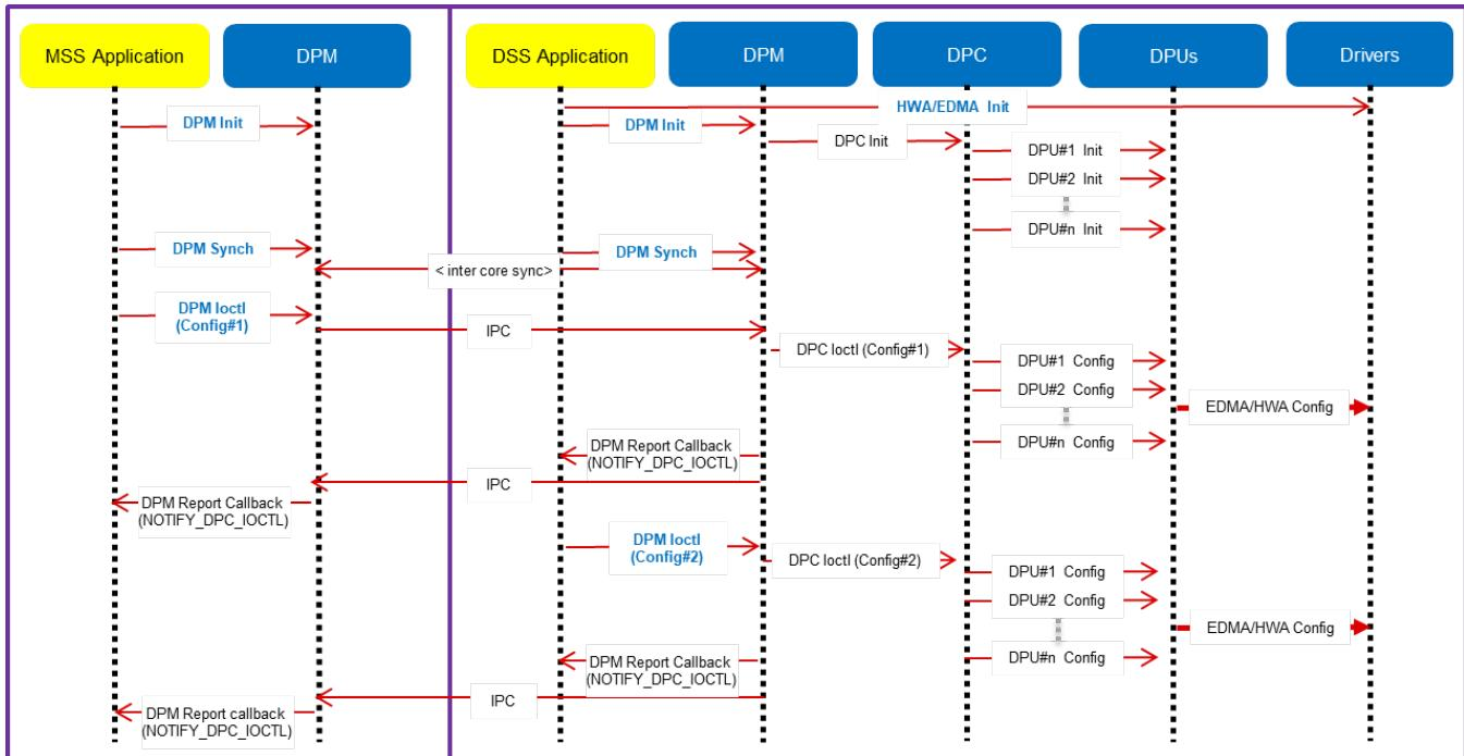
5.3.2.1 Figure 21: Data processing flow with remote domain control (init/config)
