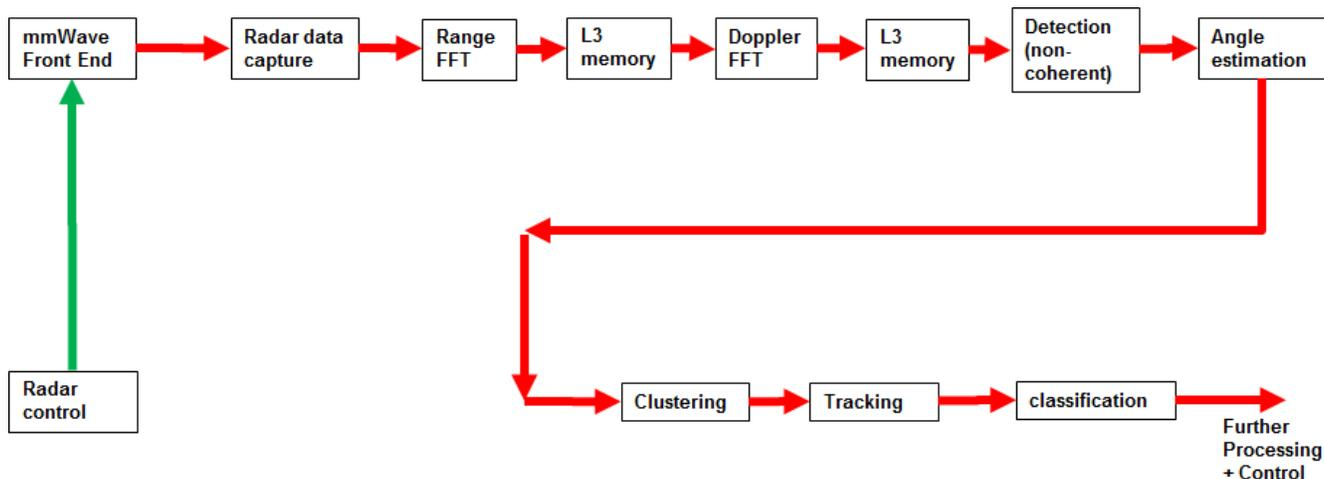
5. 2. 0. 0. 1Figure 8: Typical mmWave radar processing chain
