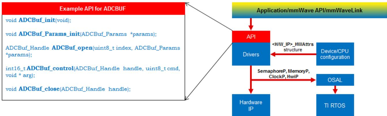
5. 4. 2. 0. 1Figure 25: mmWave SDK Drivers - Internal software design
