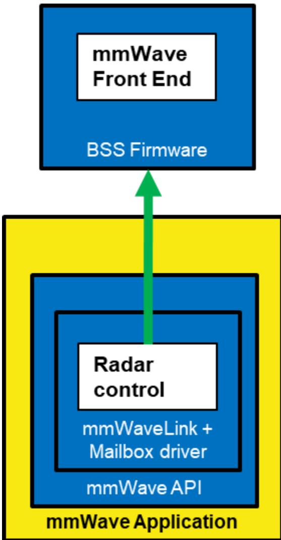
5. 3. 1. 0. 1 Figure 11: Typical mmWave radar control flow
