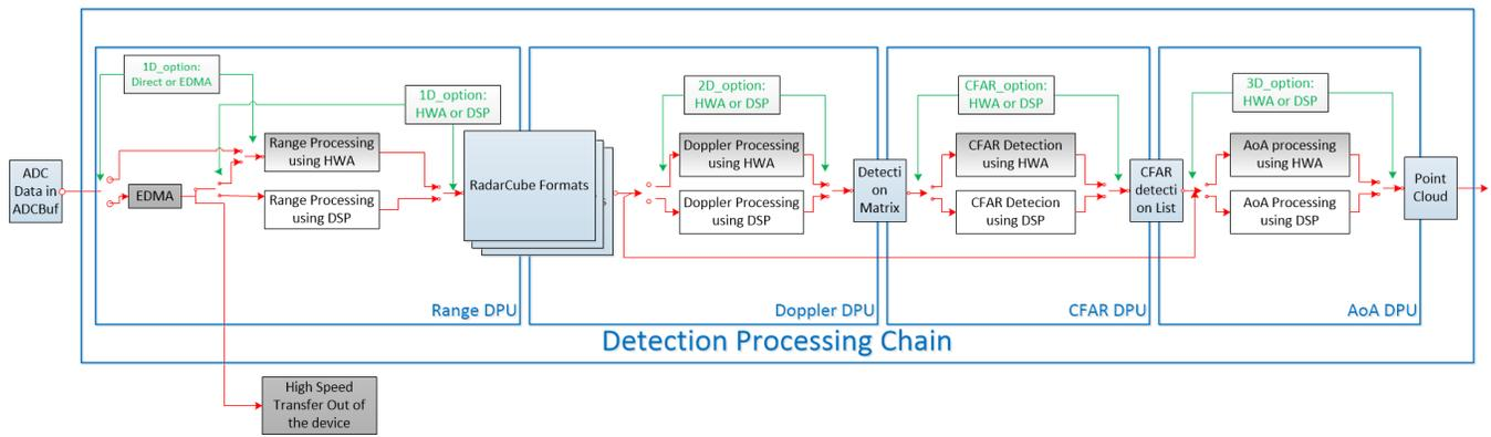
5. 2. 0. 0. 1 Figure 10: Scalable data processing chain using mmWave SDK
