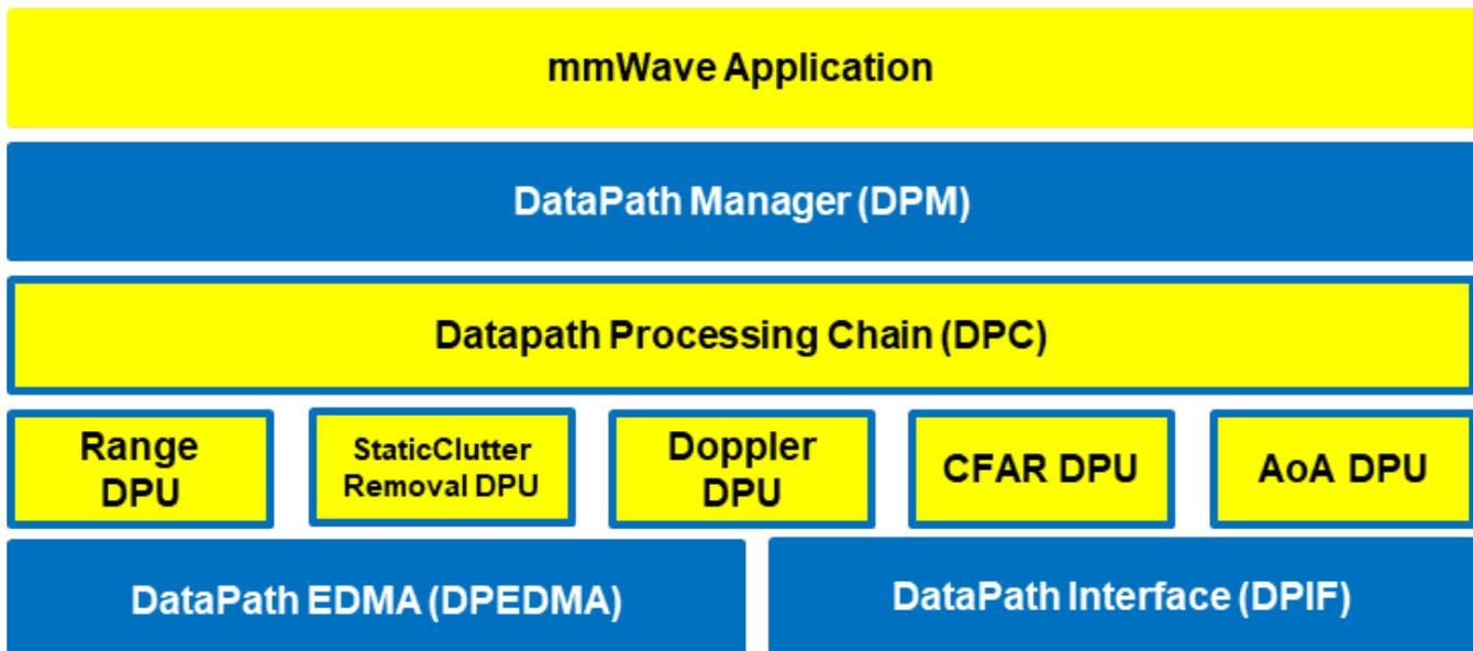
5. 3. 2. 0. 4Figure 18: Typical mmWave Detection Processing Layers
