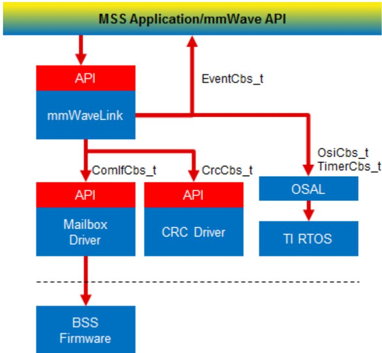
5. 4. 4. 0. 3Figure 26: mmWaveLink - Internal software design
