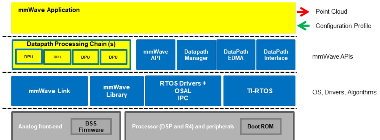
5. 1. 0. 0. 1Figure 7: SDK Layered block diagram
