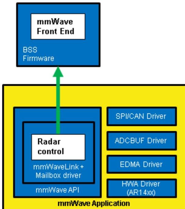
Figure 10: Typical mmWave radar control flow
