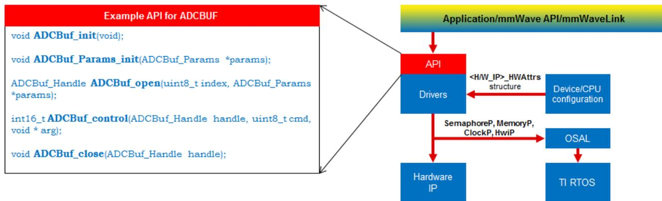
Figure 19: mmWave SDK Drivers - Internal software design
