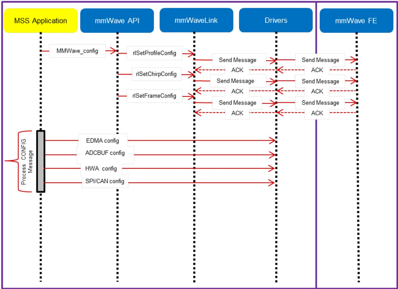
Figure 12: xWR14xx: Detailed Control Flow (Config sequence)
