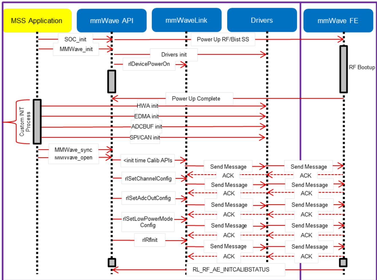
Figure 11: xWR14xx: Detailed Control Flow (Init sequence)
