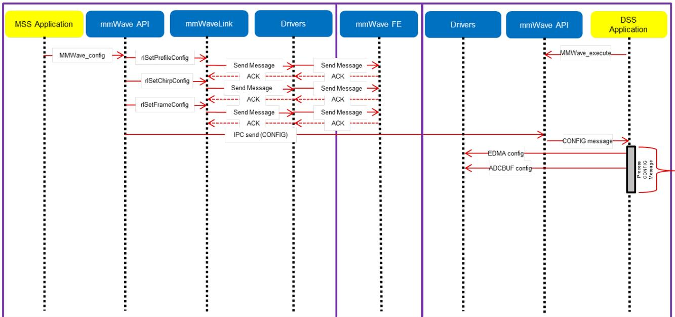
Figure 15: xWR16xx: Detailed Control Flow (Config sequence)
