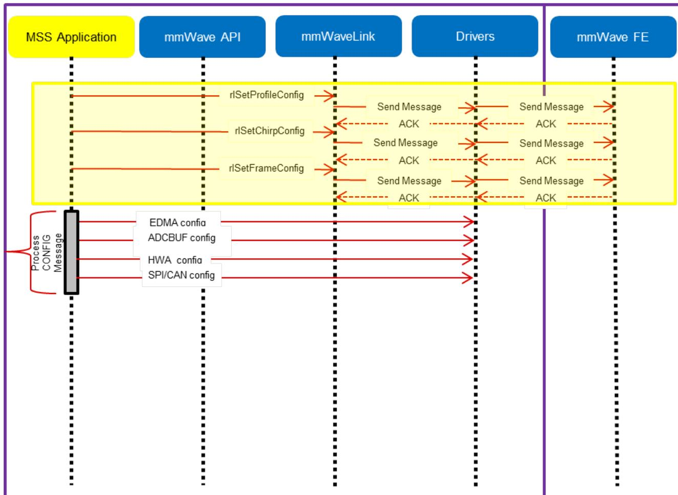
Figure 23: mmWave API - 'Minimal' Config - Sample flow (xWR14xx)
