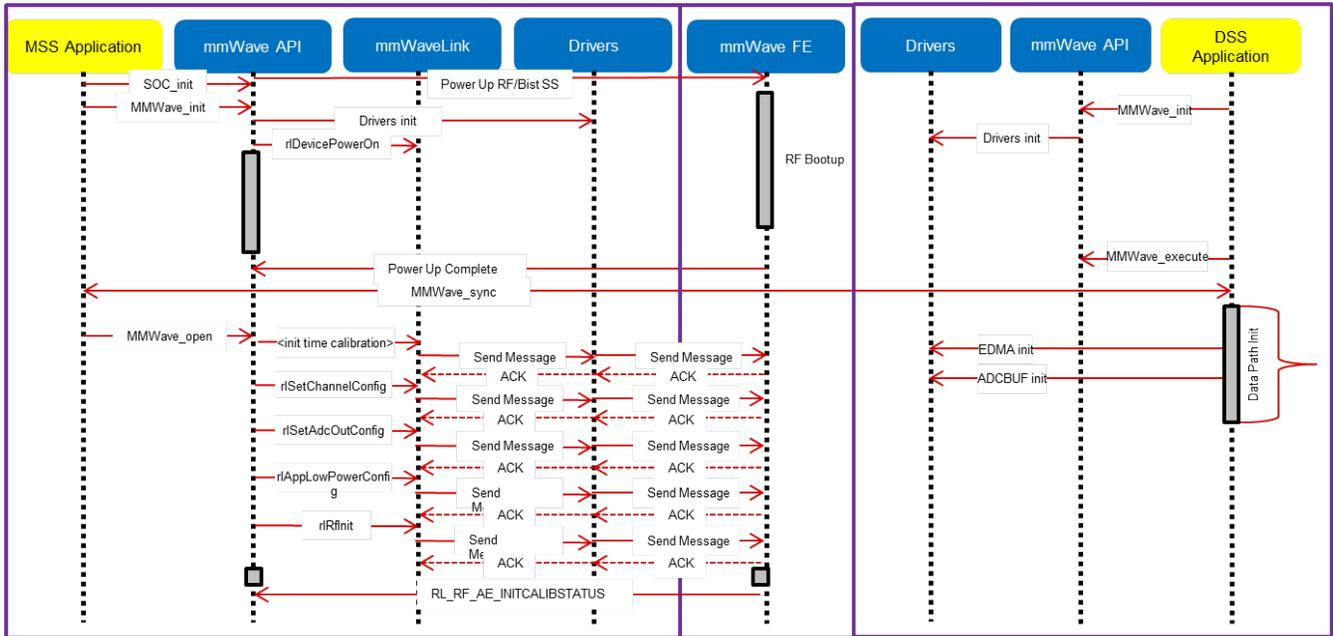
Figure 14: xWR16xx: Detailed Control Flow (Init sequence)
