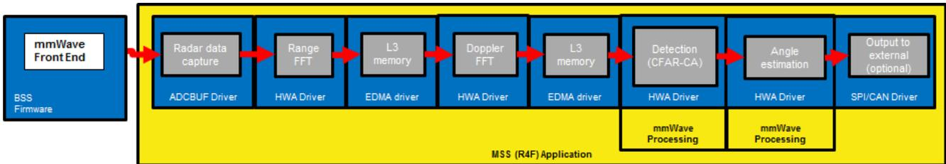
Figure 17: Typical mmWave radar data flow in xWR14xx
