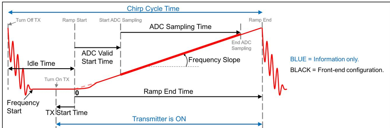
Figure 2: Chirp Diagram
