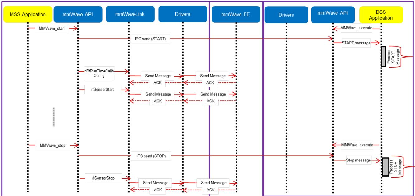
Figure 16: xWR16xx: Detailed Control Flow (Start sequence)
