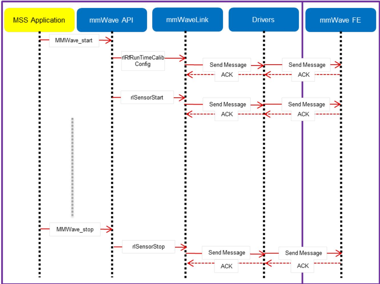
Figure 13: xWR14xx: Detailed Control Flow (start sequence)
