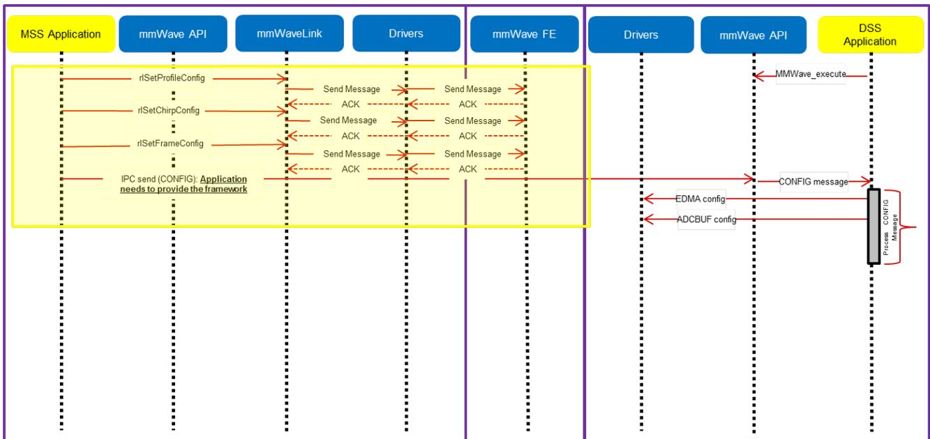
Figure 22: mmWave API - 'Minimal' Config - Sample flow (xWR16xx)
