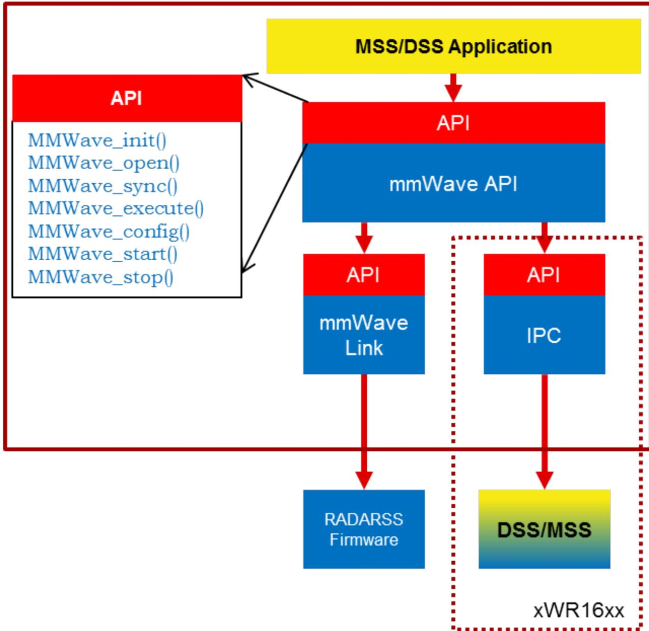
Figure 21: mmWave API - Internal software design
