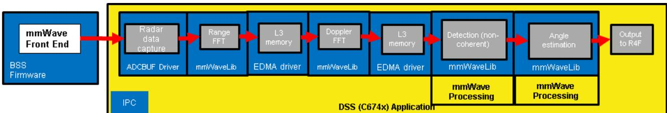
Figure 18: Typical mmWave radar data flow in xWR16xx
