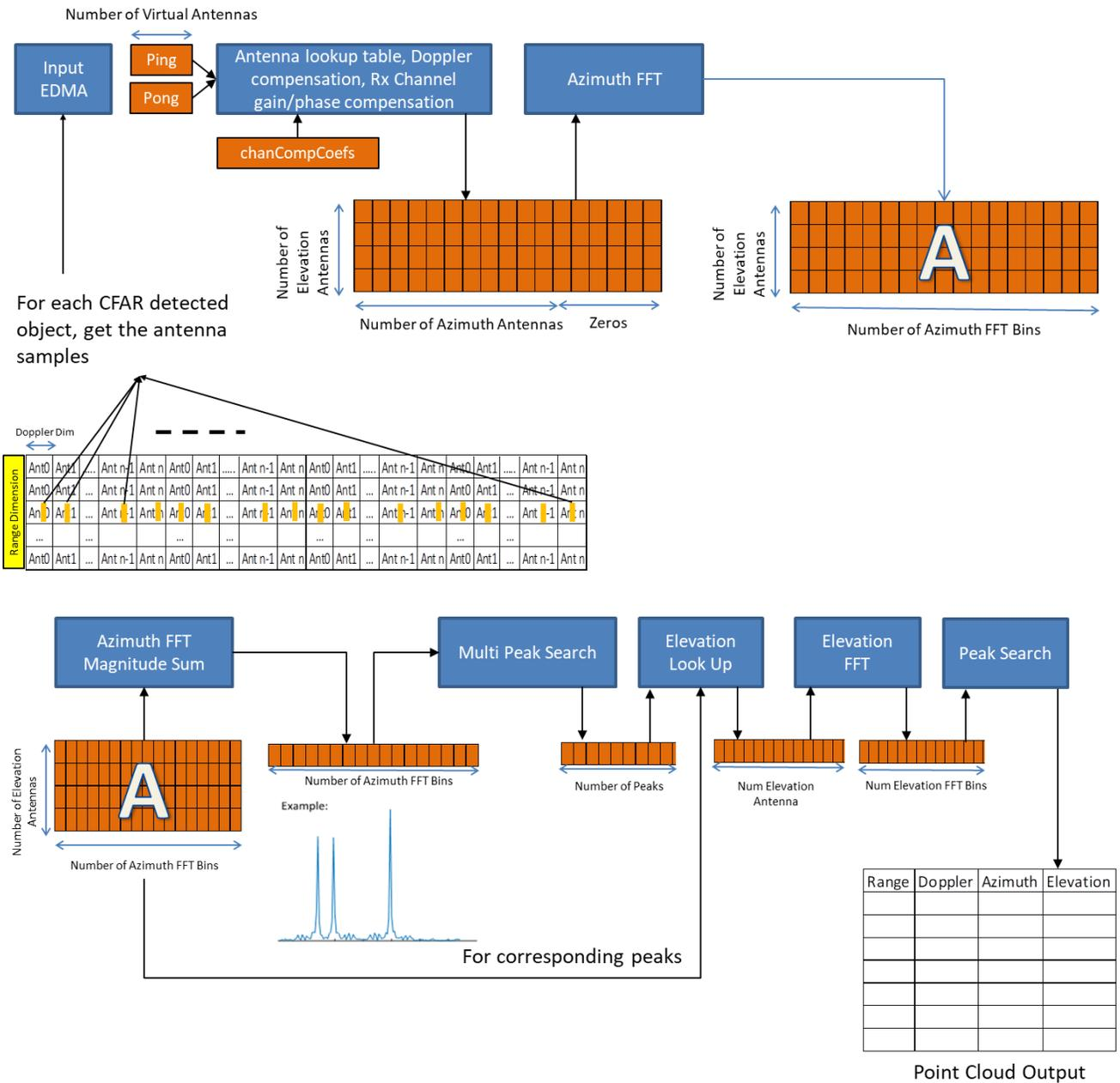
The AoA processing also includes the calibration of the compensation coefficients. The flow for the calibration is as show below:
