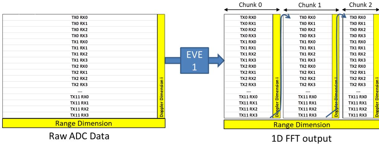
Each chunk of the EVE FFT output can be visualized as below where each Tx<sub>n</sub>Rx<sub>m</sub> pair creating a virtual Antenna (Ant).
