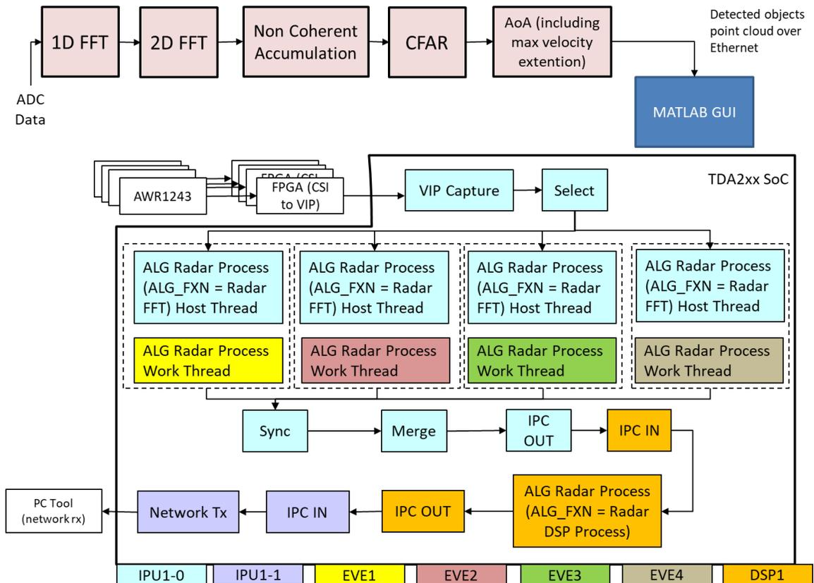
The data from the AWR1243 sensors is sent out through the CSI interface. An FPGA (LIFMD-6000) is used to convert the CSI stream to a parallel 16 bit VIP using VSYNC and ACTVID based capture. The FPGA image is capable of capturing data rates of 600 Mbps 4 Lane and 300 Mbps 4 Lane.
