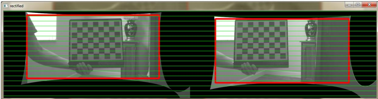
These two snapshots clearly illustrate the fact that the valid ROI red rectangles are smaller than the input image's dimensions.
