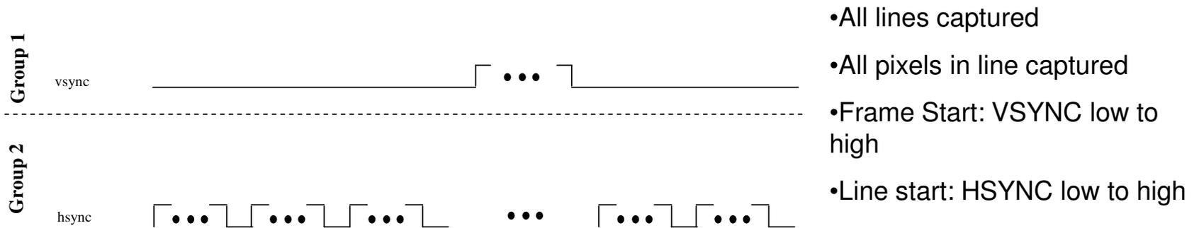
DS :Single Channel non multiplexed mode with HSYNC and VSYNC as control signals
