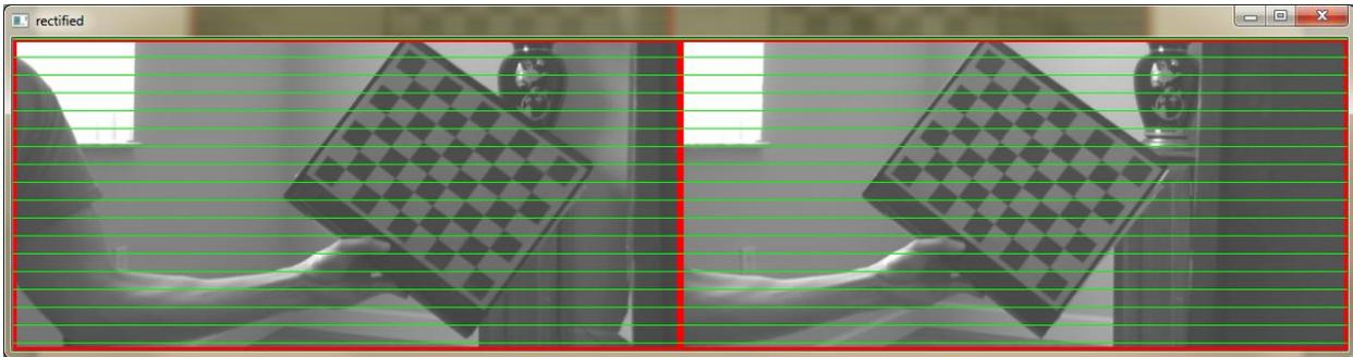
Note that a red rectangle represents a valid ROI. The snapshots above correspond to `Stereo_alpha_factor = 0`. For `Stereo_alpha_factor = 1`, we would obtain the following outputs:
