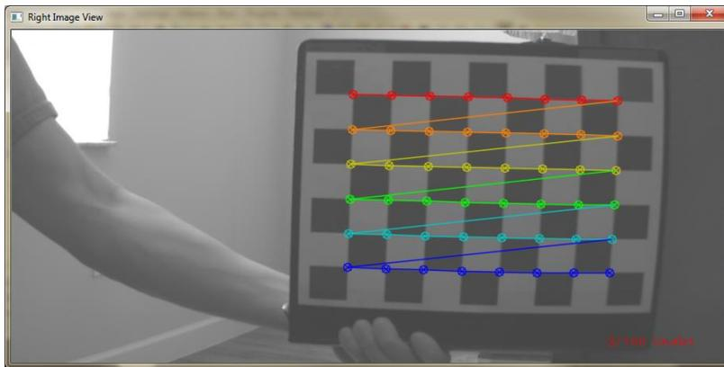
Because of the wide baseline of the monstercam' stereo cameras, there will be times where in one of the view, the checker-board pattern doesn't fit. For the lens distortion correction, since each camera is independently corrected, having unequal corner detection outcomes between left and right camera is not an issue. But later, for the stereo calibration, we need to have as many successful detected pairs as possible. Usually 2-3 undetected frames out of 10, per view, is acceptable.
