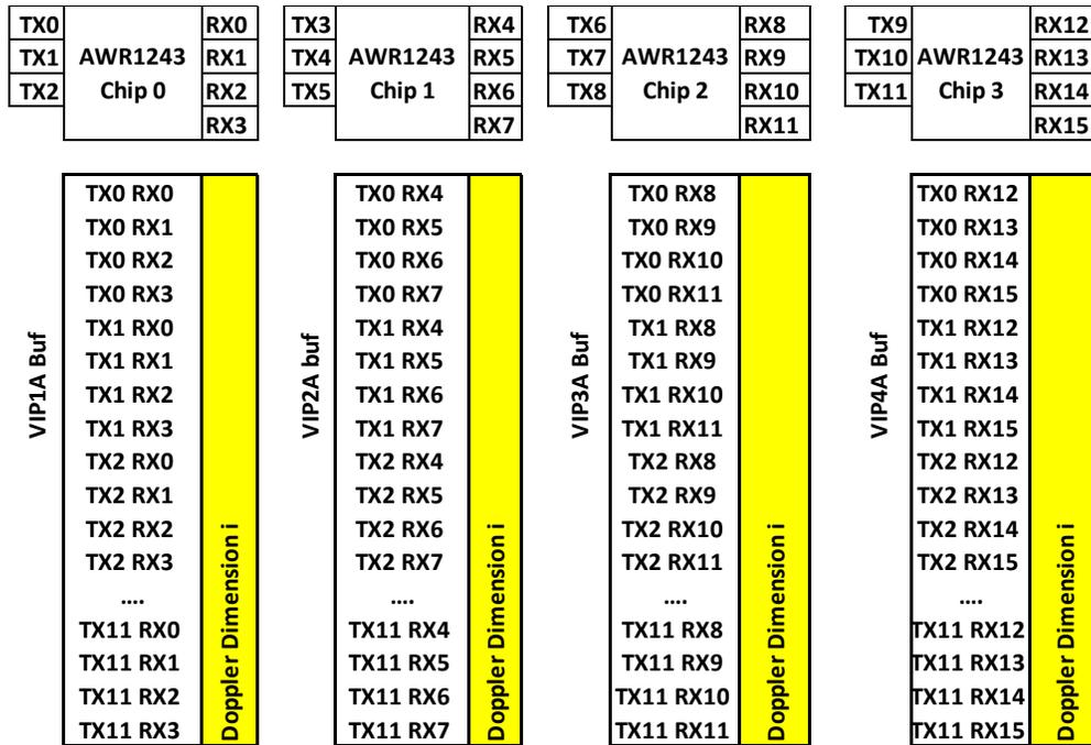
The output of each EVE 1D FFT output in DDR is as shown below:
