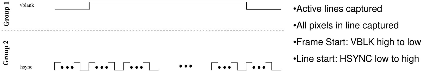
DS : Single Channel non multiplexed mode with HSYNC and VBLK as control signals
