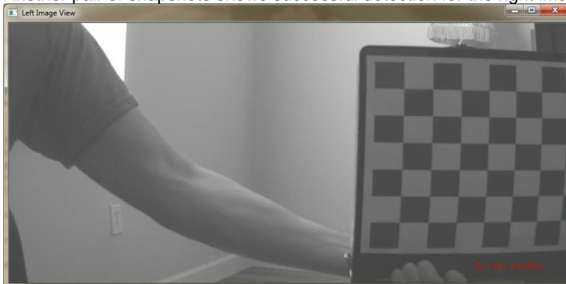
In the left view above, the checker-board is not entirely visible within the frame, causing unsuccessful detection of all the 8x6 corners.
