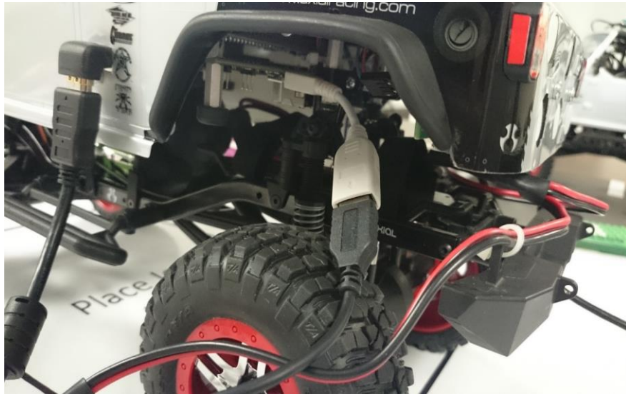
Figure 3: Connect Joystick to USB port on the EVM
