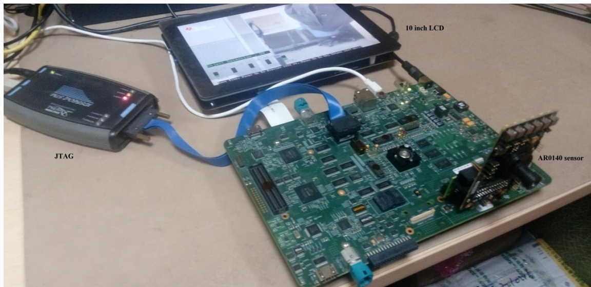
Figure: TDA3x EVM Fast boot h/w setup
