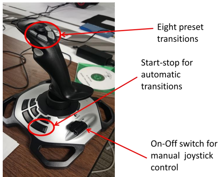
Figure 4: Preset settings on the joystick
