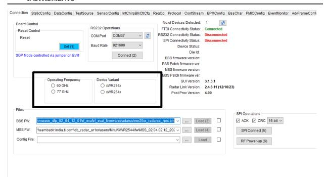
Figure 6.2. Operating Frequency and Device Variant
