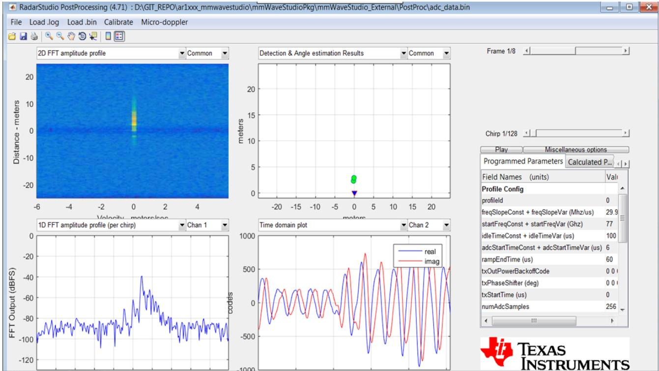
Figure 6. Visualization of the Captured Raw ADC Data
