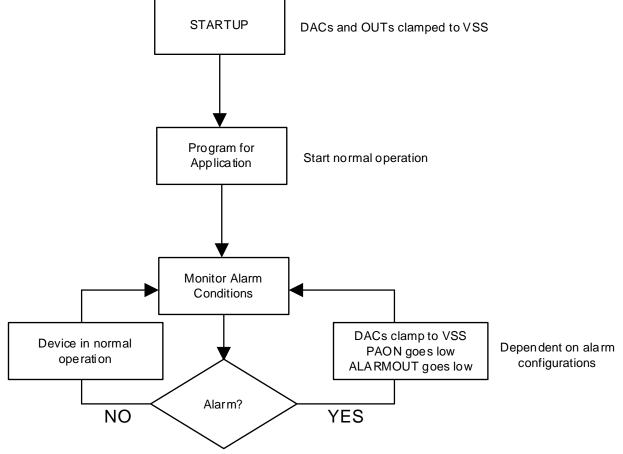
The figure is a general example of the AFE20408 operational states. When the AFE turns on, all DACs and OUTs are clamped to VSS. The device stays in this state until the AFE20408 is programmed. In the main loop, the device is monitoring all configured alarm conditions. If the AFE detects an alarm, it will set all configured DACs, OUTs, and other pins to the clamp state. The device will stay in the alarm condition until either it is cleared by the MCU or it no longer detects the alarm condition.
