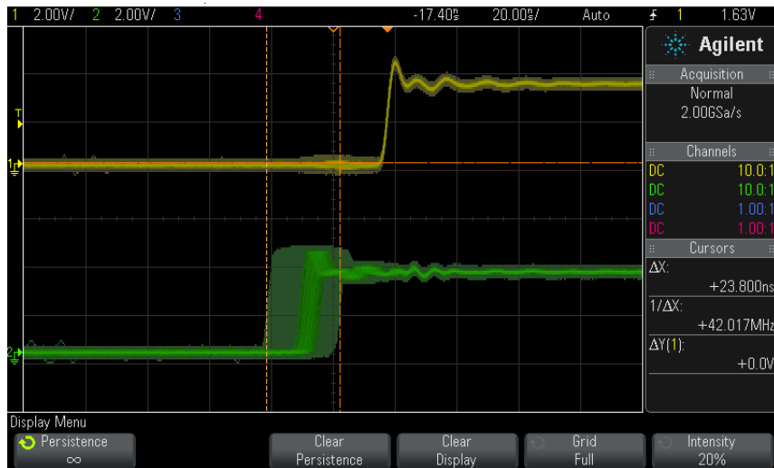
Jitter measurement oscilloscope capture after 60 hours
