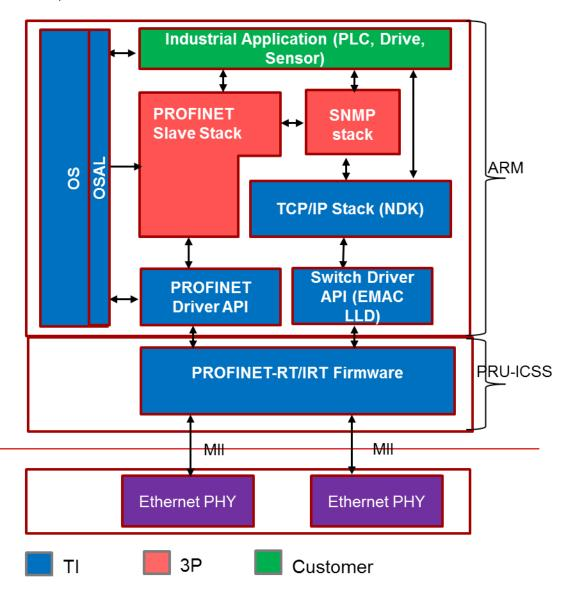
PROFINET IRT firmware for PRU-ICSS is a black box product maintained by TI. PROFINET IRT driver allows loading and run PROFINET IRT firmware and interface with the firmware.
