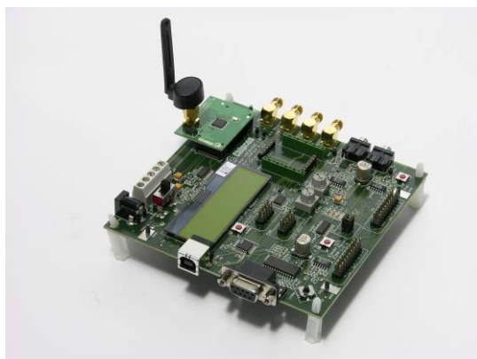
Figure 1: A SmartRF ® 04EB with a CC2510EM and antenna
