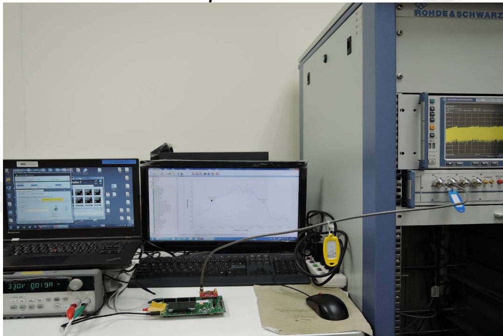
Test Set up Photos – Conducted
