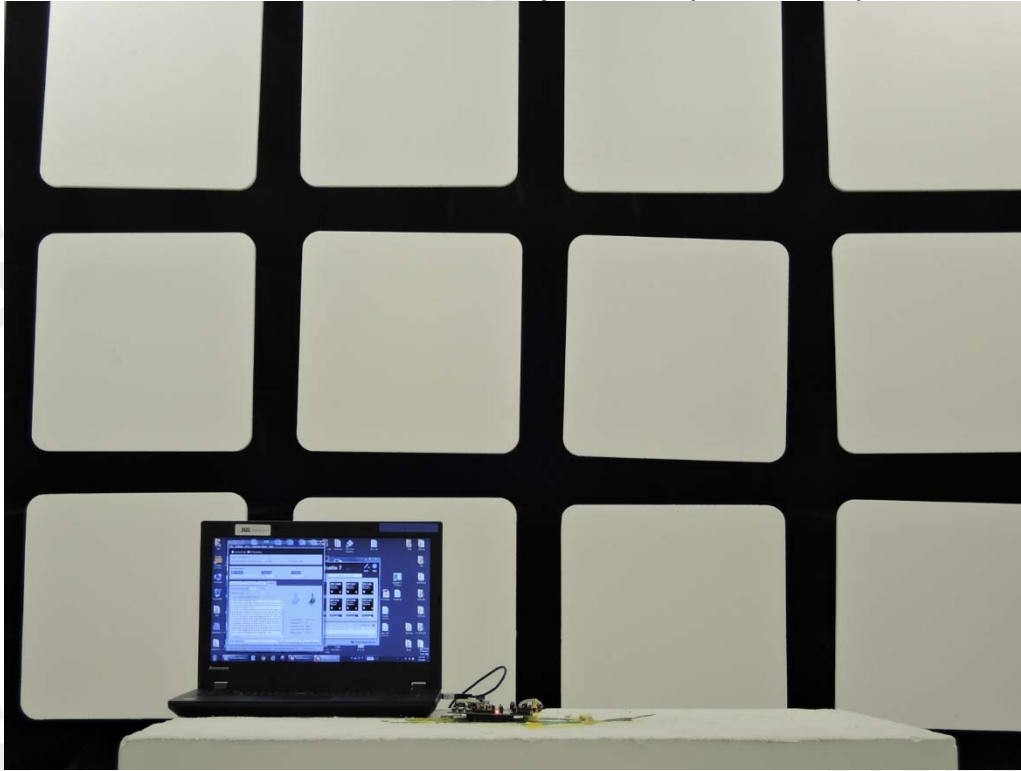
Radiated Emission Set up Photos (Front View)
